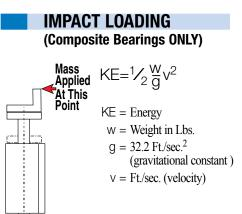
In applications such as conveyor stops impact loading may be a factor. The table below gives the maximum KE energy for each of the PB2 models. Use the above equation to determine the KE for your application. Your result should not exceed the maximum KE for the PB2 model you select.
