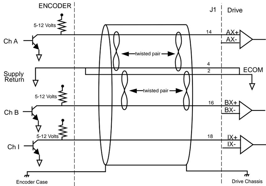
Figure 6.28 Single-Ended Encoder Interface via Open Collector Transistor with 5 VDC to 12 VDC Pull-up
