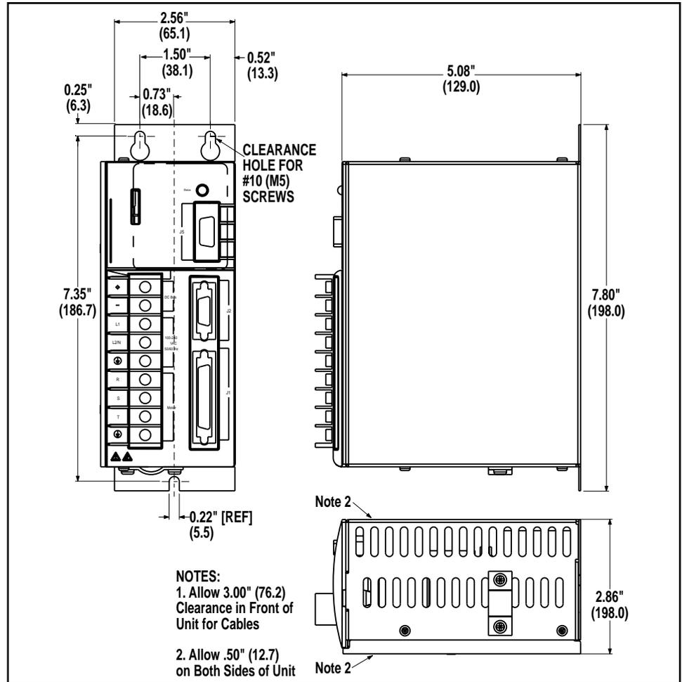
Figure 5.1 SSD5 Mounting Dimensions
