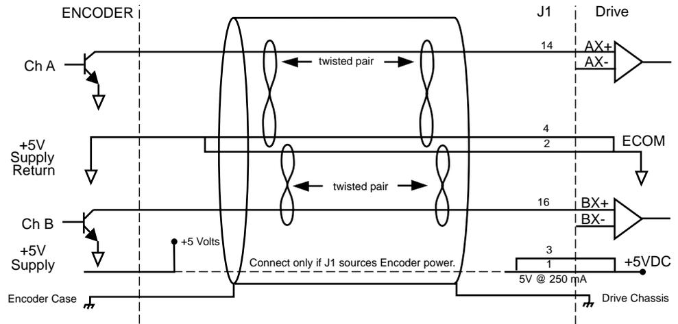
Figure 6.26 Single-Ended Encoder Interface via Open Collector Transistor without Pull-up
