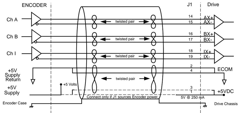
Figure 6.23 External Encoder Interface via TTL Differential Line Drivers
