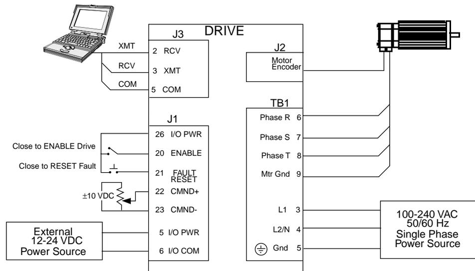
Figure 8.1 Analog Controller Connection Diagram
