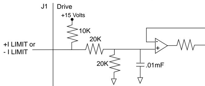
Figure 6.17 External Current Limit Circuit
