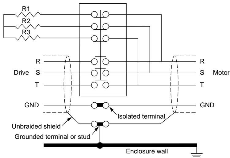
Figure 7.1 Emergency Stop Contractor Wiring
