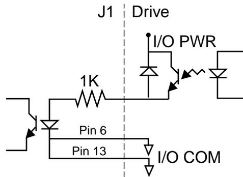
Figure 6.10 Drive Output Connected to an Opto-Isolator
