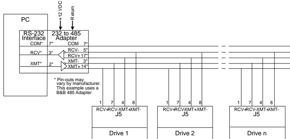
Figure 6.40 RS-232 to RS-485 Multi-Drop Connection Diagram
