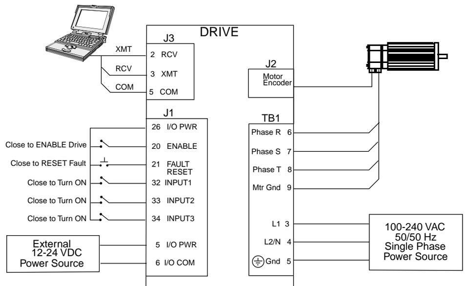
*Figure 8.2 Preset Controller Connection Diagram*
