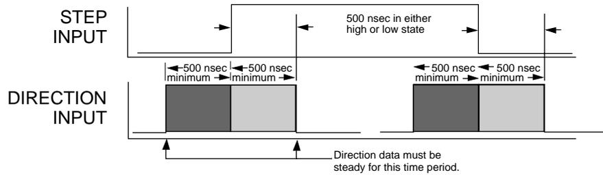
Table 6.S Step/Direction and CW/CCW (Step Up/Step Down) Interface Specifications
