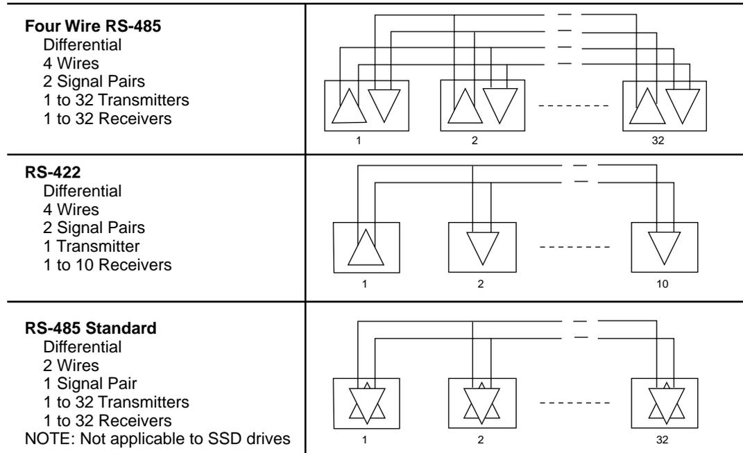
Figure 6.39 RS-485/RS-422 Communication Comparison
