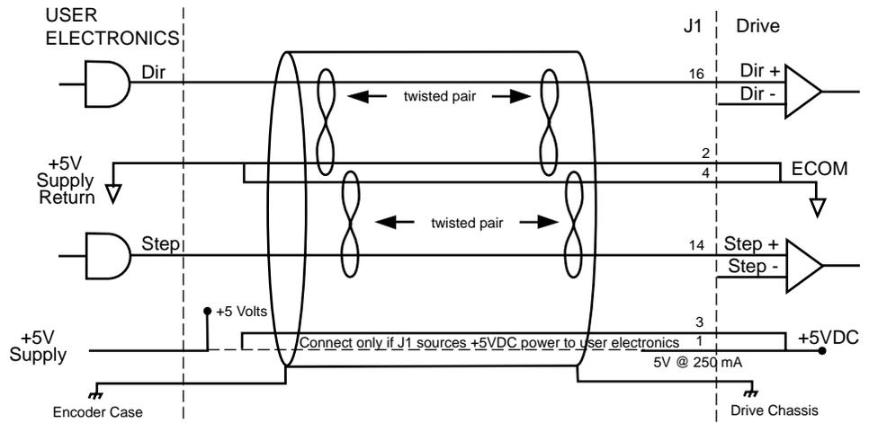
Figure 6.31 External Step/Direction Interface via Single-Ended TTL Line Drivers
