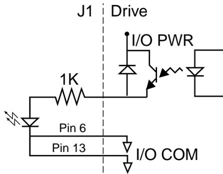
Figure 6.12 Drive Output Connected to a Resistive Load
