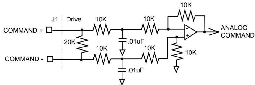
Figure 6.18 Analog COMMAND Input Circuit
