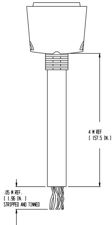
Figure B.2 J1 Connector to Flying Leads
