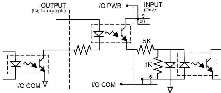
Figure 6.6 Drive Input Connected to Active Low Output using an Opto-Isolator
