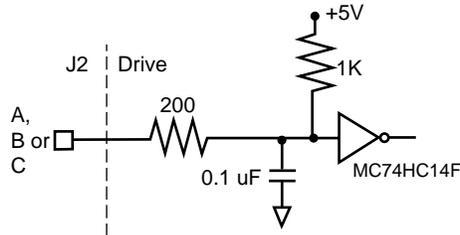
Figure 6.35 Hall Effect Sensor Circuit
