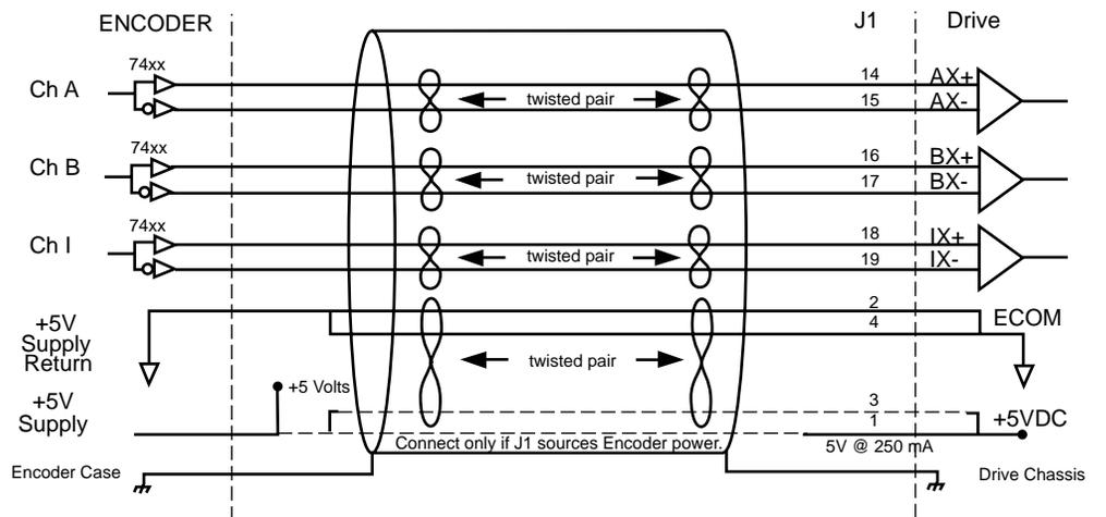
Figure 6.25 Complementary Encoder Interface via Standard TTL Logic
