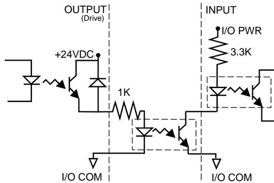
Figure 6.15 Drive Output Connected to Active Low Input using an Opto-Isolator
