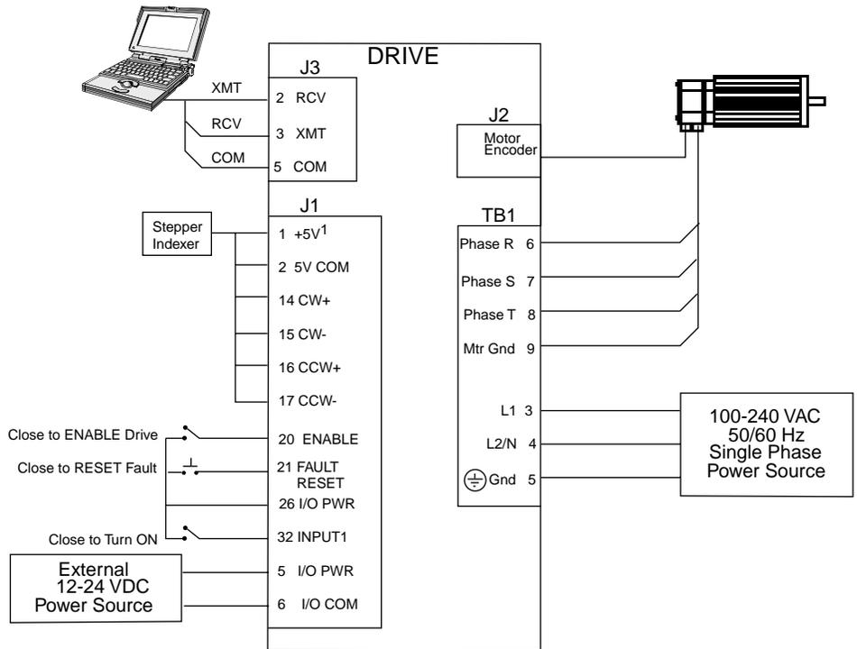
*Figure 8.5 Position Follower (Step Up/Down Controller) Connection Diagram*
