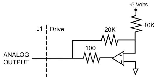
Figure 6.19 ANALOG 1 Output Circuit
