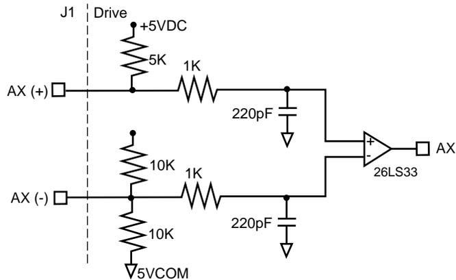
Figure 6.22 Auxiliary Encoder Input Circuit
