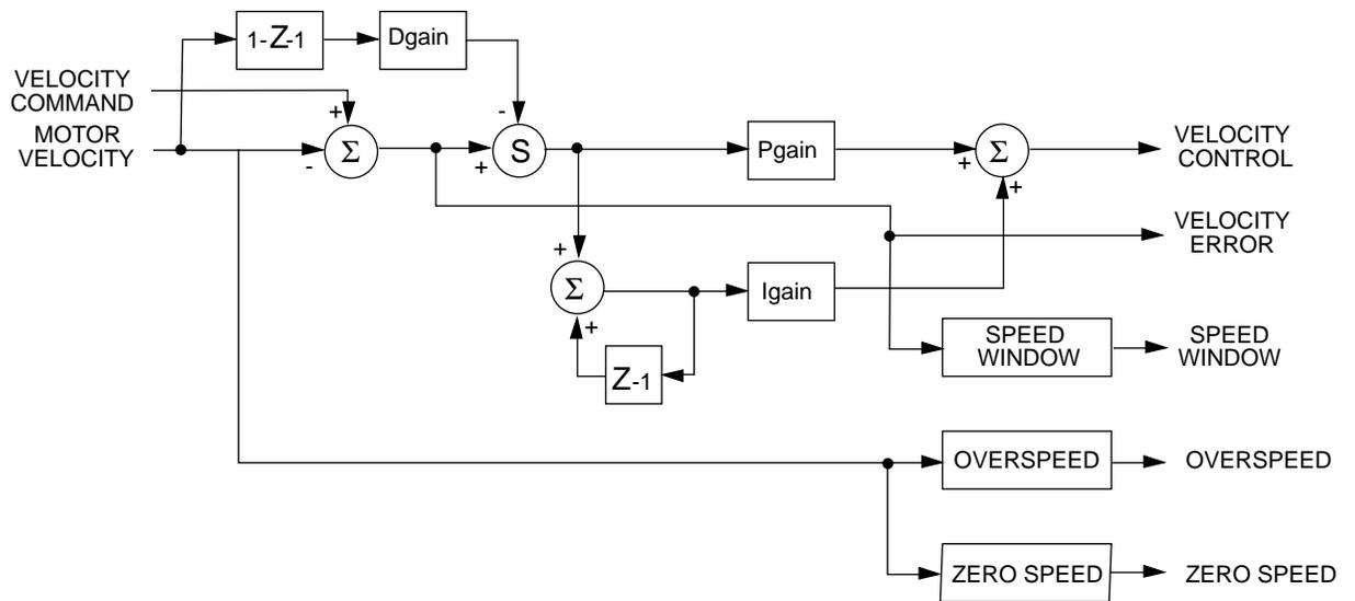
Figure 9.1 Velocity Loop Structure
