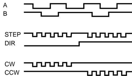
*Figure 6.21 Auxiliary Encoder Inputs*
