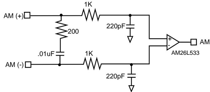
Figure 6.34 Motor Encoder Interface Circuit
