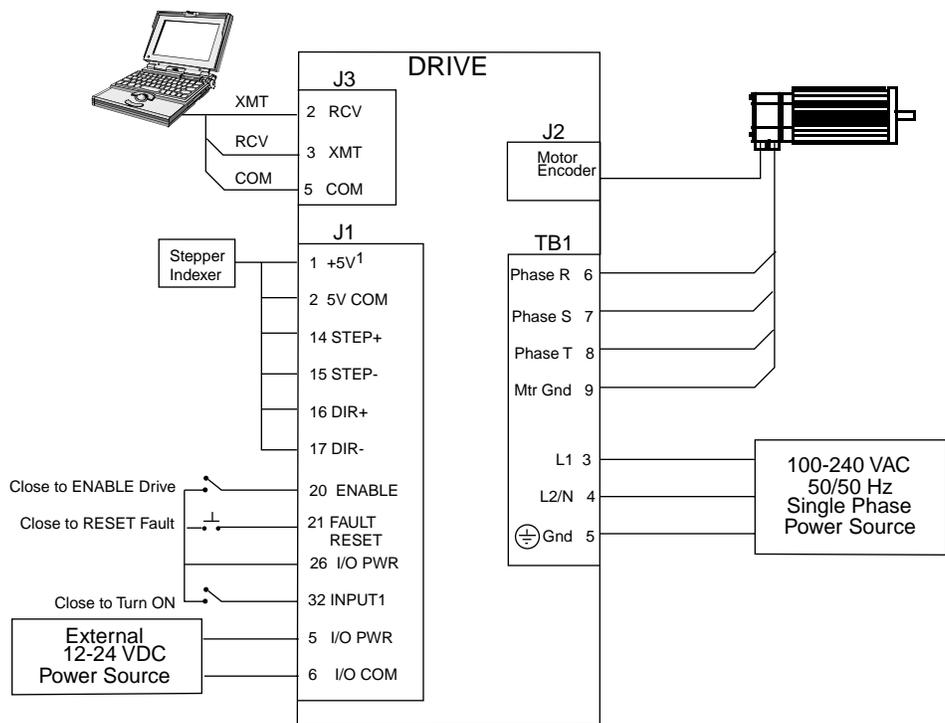
Figure 8.4 Position Follower (Step/Direction Controller) Connection Diagram
