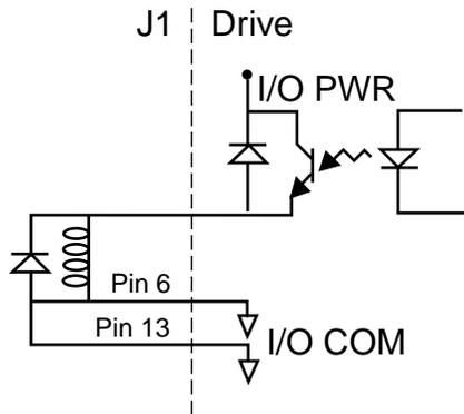
Figure 6.13 Drive Output Connected to a Switch/Relay
