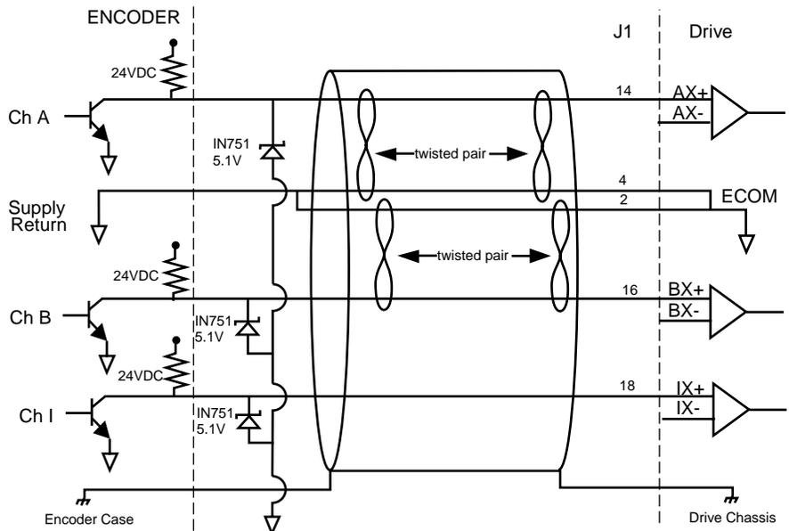
Figure 6.29 Single-Ended Encoder Interface via Open Collector Transistor with 24 VDC Pull-up
