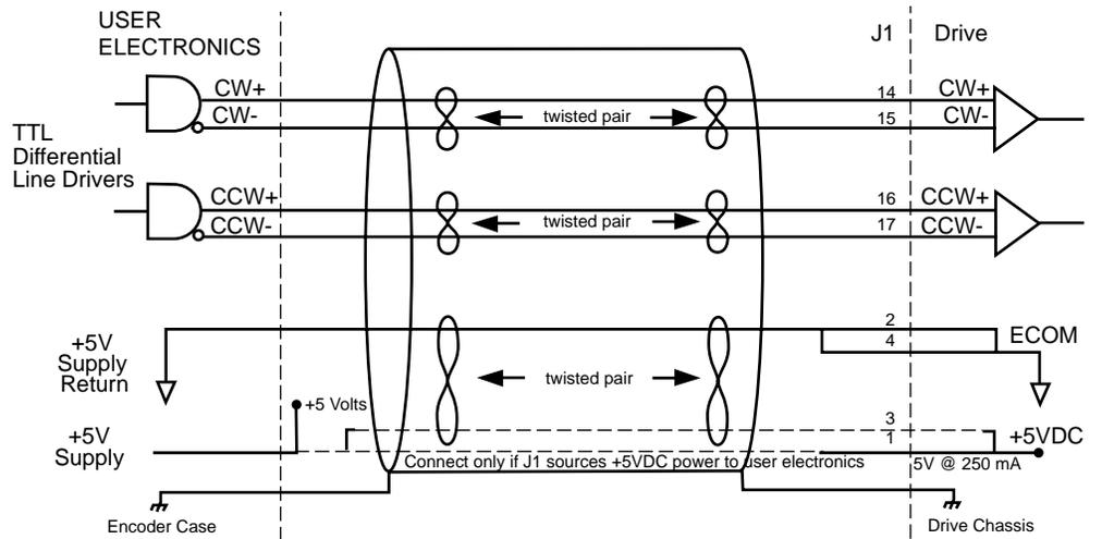
Figure 6.32 External CW/CCW (Step Up/Step Down) Interface via TTL Differential Line Drivers
