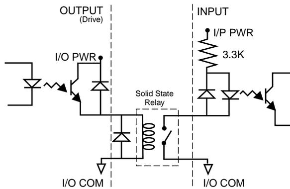
Figure 6.14 Drive Output Connected to Active Low Input using a Switch/Relay
