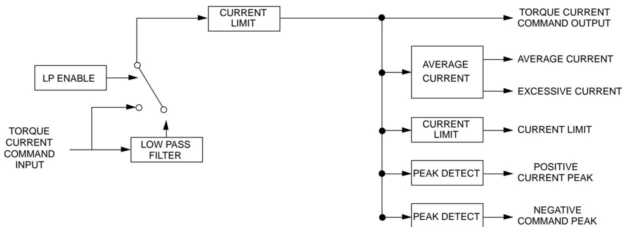
Figure 9.2 Torque Current Conditioning Structure
