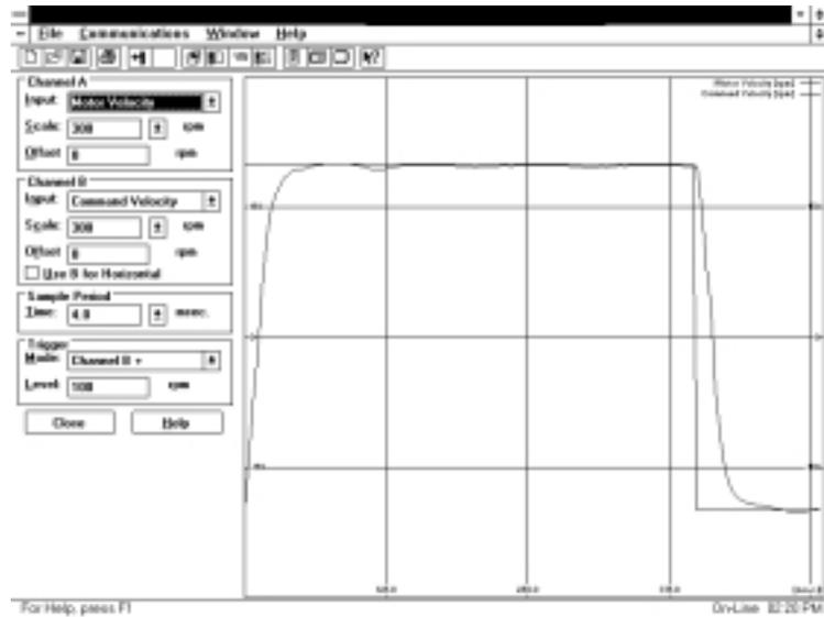
Figure 9.5 Overdamped Signal
