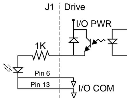
Figure 6.11 Drive Output Connected to an LED Indicator
