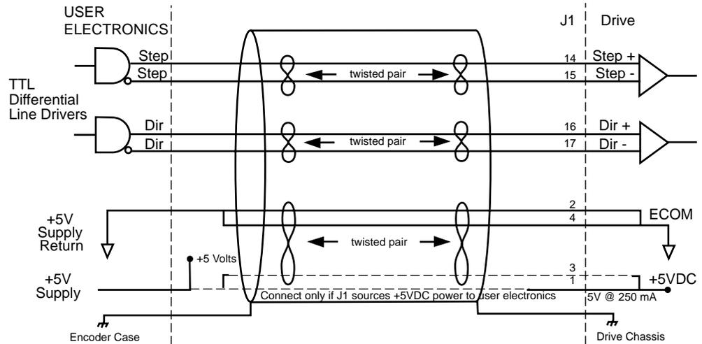
Figure 6.30 External Step/Direction Interface via TTL Differential Line Drivers
