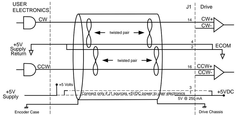
Figure 6.33 External CW/CCW (Step Up/Step Down) Interface via Single-Ended Line Drivers
