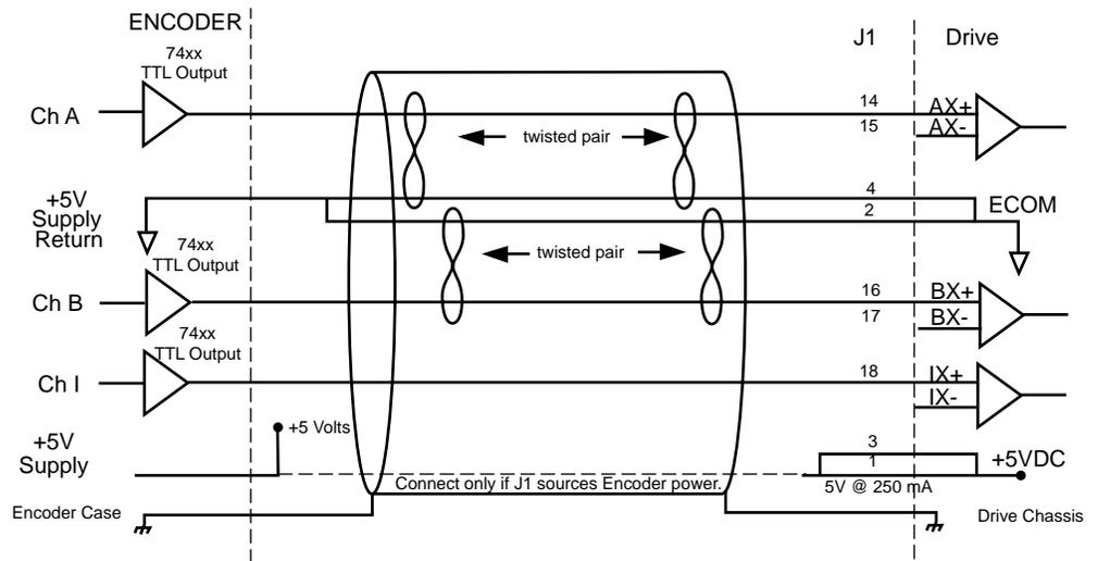
Figure 6.27 Single-Ended Encoder Interface via Standard TTL Signals
