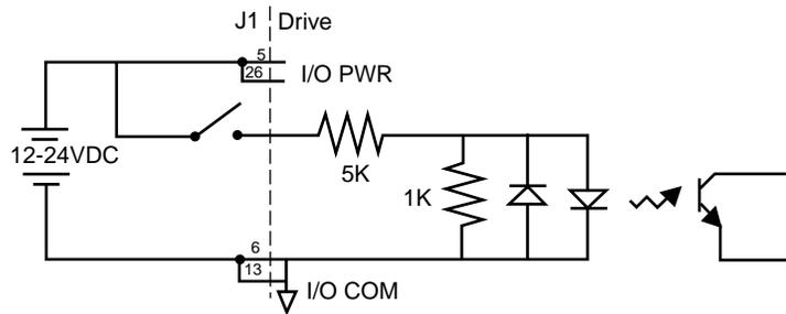
Figure 6.2 Drive Input Connected to a Switch/Relay Contact
