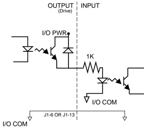
Figure 6.16 Drive Output Connected to Active High (Sinking) Input
