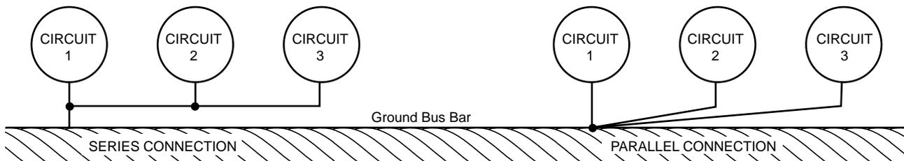
Figure C.3 Single Point Ground Types
