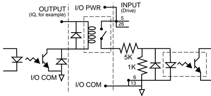
Figure 6.5 Drive Input Connected to Active Low Output using a Switch/Relay
