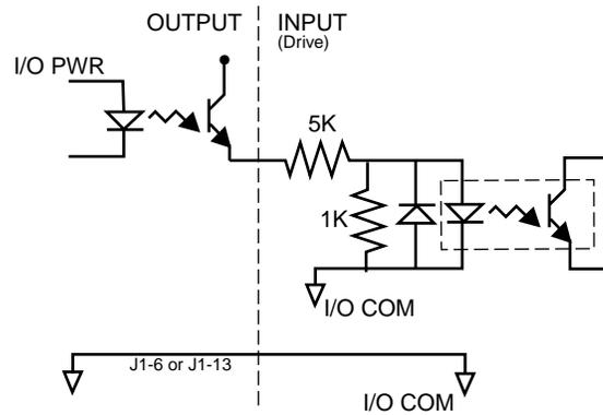
Figure 6.7 Drive Input Connected to Sourcing Output
