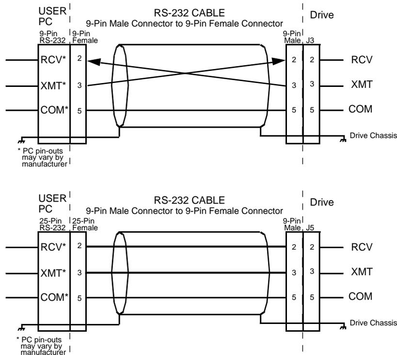
Figure 6.38 RS-232 Connection Diagrams
