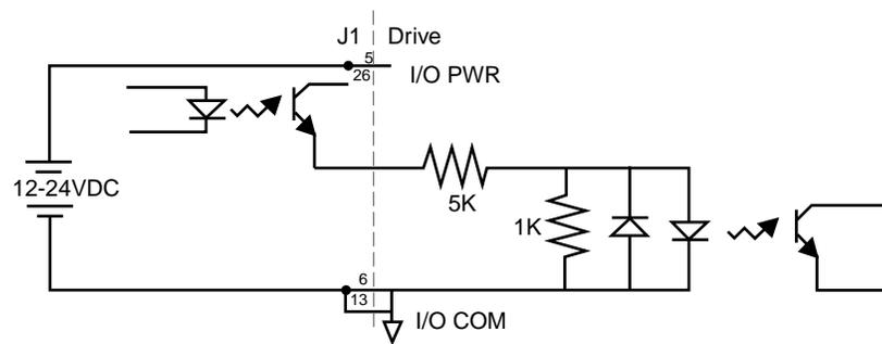
Figure 6.3 Drive Input Connected to an Opto-Isolator
