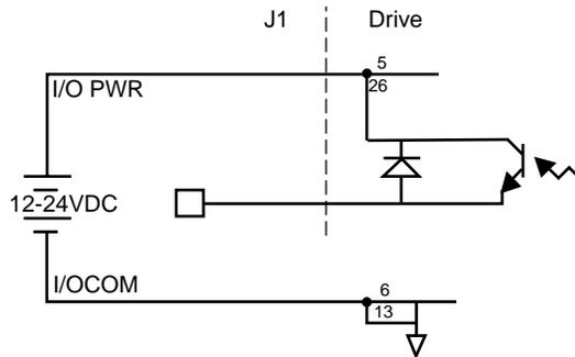
Figure 6.9 Digital Output Circuit.
