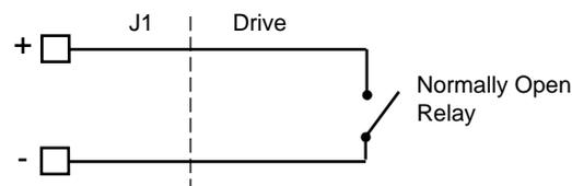
Figure 6.8 READY and BRAKE/DRIVE ENABLED Circuits
