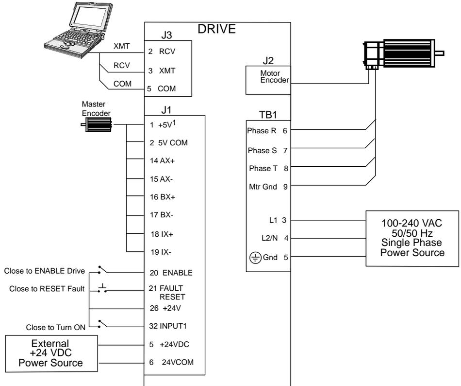
Figure 8.3 Position Follower (Master Encoder) Connection Diagram
