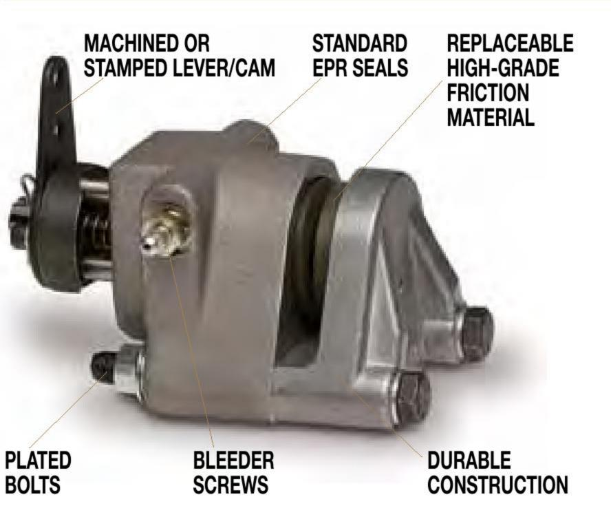
These Tolomatic brakes combine hydraulic and mechanical braking in one caliper. Available in the H/ME20 Series and H/ME220 Series these single acting calipers deliver high braking torque in a small package. Features include: replaceable, high-grade friction material, standard EPR seals, aluminum or cast iron construction (depending on model), bleeder screws and zinc plated bolts. Options include Buna-N seals, Viton® seals and floating brackets. (See pages 50 to 55)
