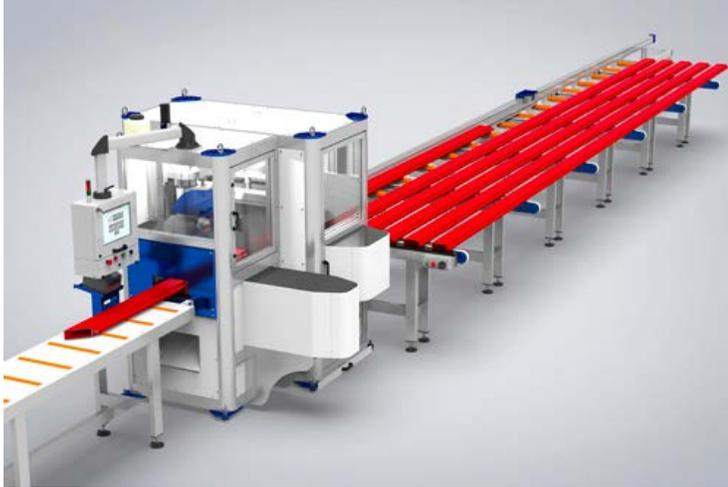
*The 9-axis RhinoFab glazing machine, which pre-drills and cuts lineal materials to spec, is designed to deliver the required force and pressure to drill perfectly placed holes and route intricate patterns.*
