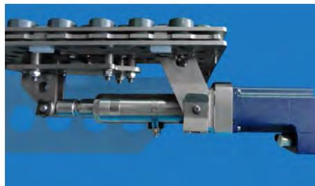
As the Tolomatic ERD actuator moves in and out, it activates the center plate above that rotates the cams on the top plate. These cams, in turn, activate rollers in the moving belt to create lateral movement.
