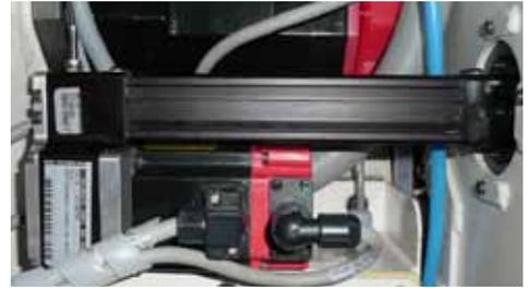
Tolomatic's RSM actuator features a reverse-parallel motor drive with the motor mounted along side the actuator, driving the screw through a toothed belt and pulley assembly. The compact actuator series is designed for high-performance thrust from 70 to 7,000 pounds, accuracy and durability.
