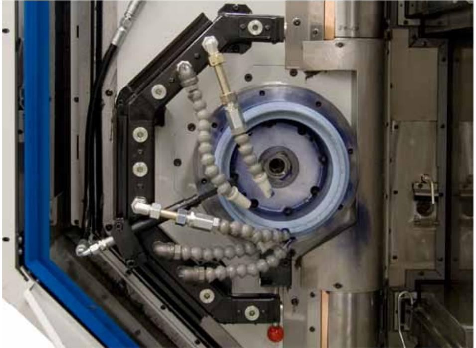
The heavy, C-shaped coolant manifold on the Phoenix II 275G gear grinding machine is moved incrementally by a Tolomatic RSM actuator as the circular grinding wheel wears away. This keeps the coolant flow precisely directed at the point of contact with the gear face.
