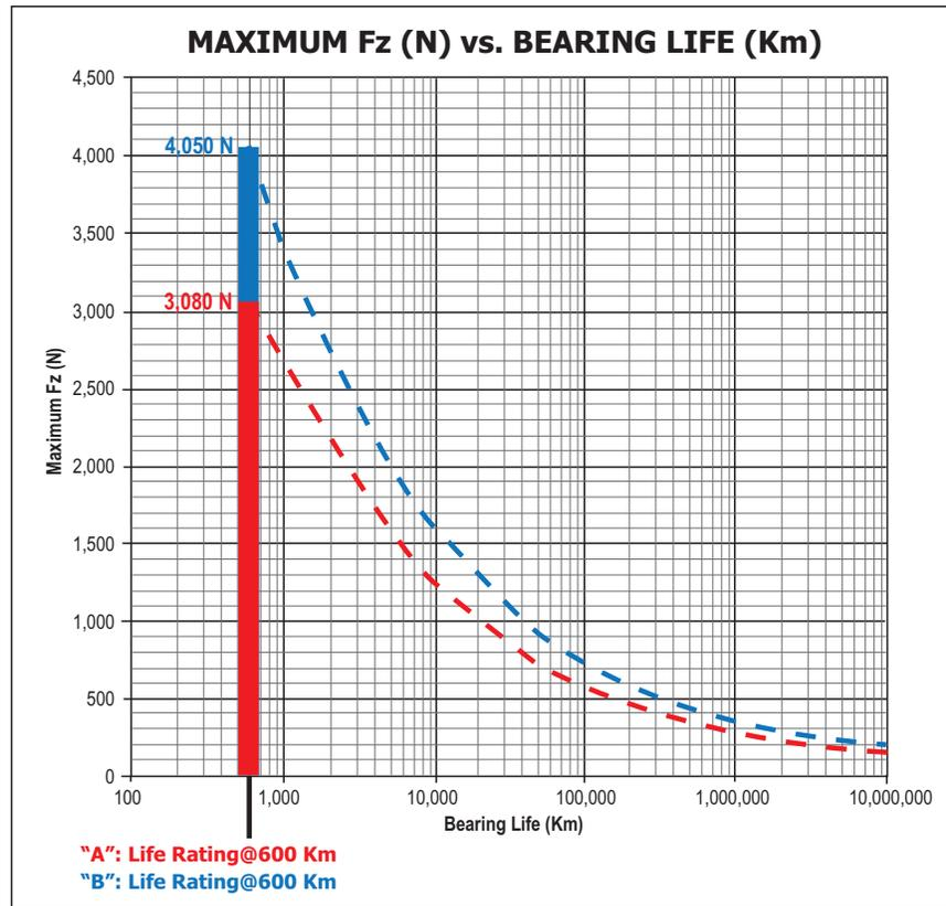
Evaluating both actuators based on the distance they are expected to travel in service at the same life ratings reveals that manufacturer "B" product will, for a given load, travel approximately 100% farther. This translates into longer useful service life and is clearly the stronger more robust product.
