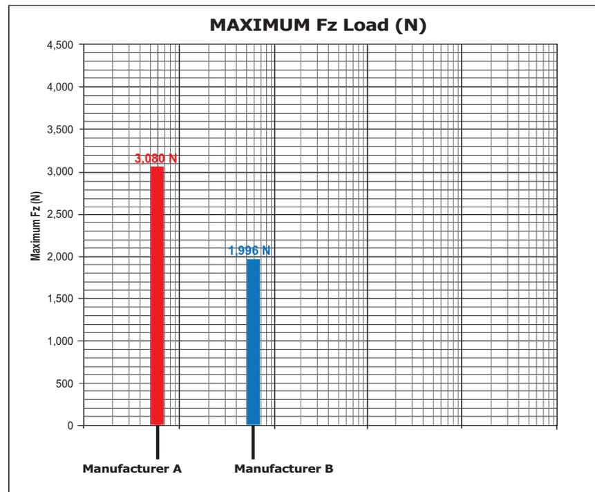
Based only on the highest value, it appears to be manufacturer "A." However, additional investigation reveals what the load rating really means. Since load ratings are to be based on the L10 life of bearing travel, we need to determine the distance of travel for which the maximum loads are rated.
