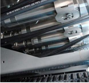
When determining the life of an actuator, inside a machine application, it is important to evaluate the effects of loading on the screw. Calculating for constant loads requires a different formula than calculating for varying loads. Besides load, other factors affect how the screw performs inside the actuator, including manufacturing methods, actuator design, lubrication, velocity, temperature, wear, corrosion, contamination and other dynamic elements such as misalignment and vibrations.
