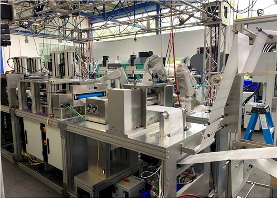
*The workcell is designed so it can be adapted to make masks for a variety of medical procedures. Shown: Mask workcell material infeed and transfer station. Photo: Tolomatic, Inc.*
