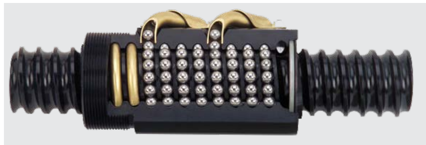
Ball screws are ideal for low-duty-cycle applications with moderate force requirements and moderate to high speeds. A ball screw's ball bearings have fewer points of contact than roller screws, resulting in a lower life expectancy.
