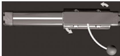
The same thing happens when the cylinder cycles to the other end of stroke. The resultant dynamic moment may exceed the rated capacity of the actuator. After repeated cycles, the actuator may not achieve its designed life expectations if not properly selected.
