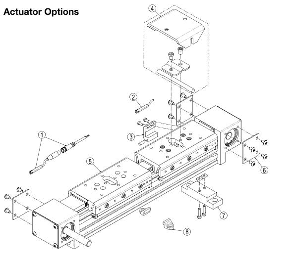
**To order service parts switches:** Switches for MXB include retained mounting hardware and are the same for all actuator sizes and bearing styles
