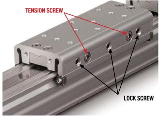
engage. The Carrier will be loose but should not rock sideways. To correct this, loosen the Lock Screws about 1/16 of a turn. If the Carrier becomes too snug, adjust the Lock Screws another 1/8 of a turn.
