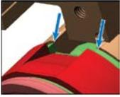
Verify surface of Piston is behind the surface of the Piston Bracket in both places as shown in diagram.
