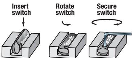
Place switch in side groove on tube at desired location with "Tolomatic" facing outward. While applying light pressure to the switch, rotate the switch halfway into the groove. Maintaining light pressure, rotate the switch in the opposite direction until the switch is fully inside the groove with "Tolomatic" visible. Re-position the switch to the exact location and lock it securely into place by tightening the screw on the switch.
