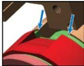
Verify surface of Piston is behind the surface of the Piston Bracket in both places as shown in diagram.
