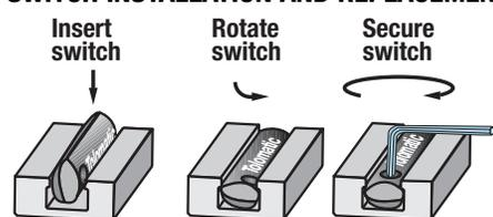
Place switch in side groove on tube at desired location with "Tolomatic" facing outward. While applying light pressure to the switch, rotate it such that the switch is halfway in the groove. Maintaining light pressure, rotate the switch in the opposite direction until the switch is fully inside the groove with "Tolomatic" visible. Re-position the switch to the exact location and lock the switch securely into place by tightening the screw on the switch.
