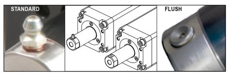
Figure 7.1: A standard or a flush style grease zerk allow periodic relubrication for the GSWA33, 04, 44 & 55 actuator. This can often be done without removing the actuator from its installation.
