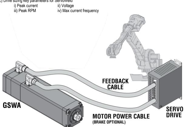
Figure 4.1: Typical connections for a single-axis system with an ServoWeld<sup>™</sup> actuator with optional brake to a RSW servo system drive
