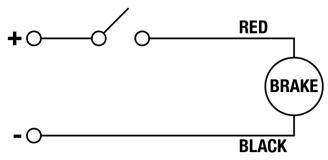
Figure 6.1: Fastest Engage / Disengage time, least protection
