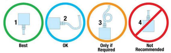
Figure 5.1: Recommended routing of ServoWeld cabling.
