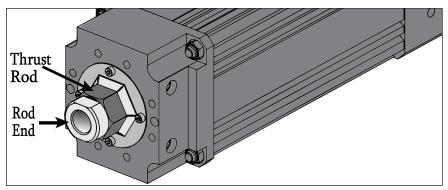
Figure 4.5: The hexagonal shape of the GSWA04 thrust rod does not allow the rod to rotate but does not provide guidance of the load.
