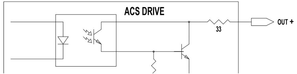
**Figure 6-6: Output Circuit**
