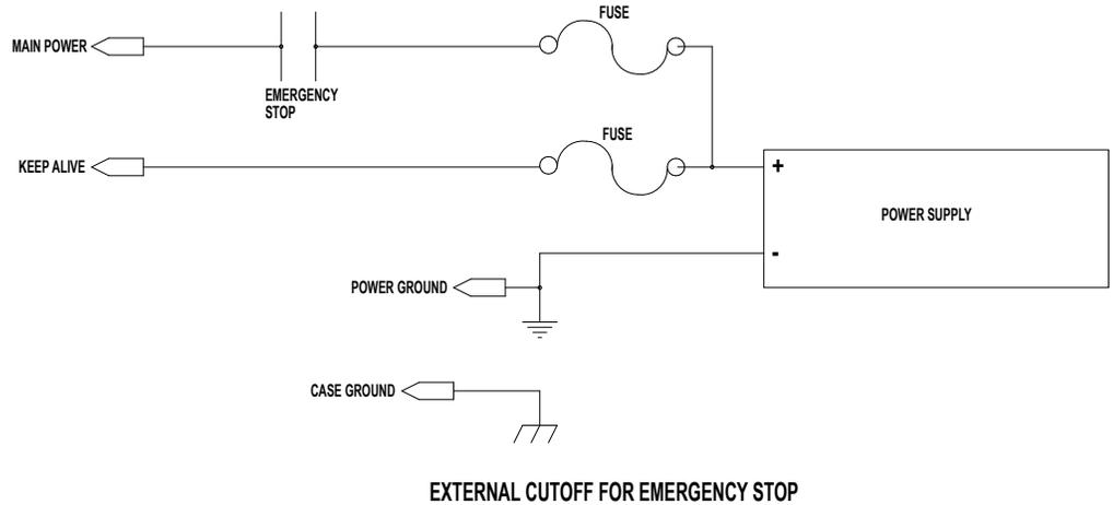
**Figure 6-13: ACS Drive External Cutoff Switch for Emergency Stop**
