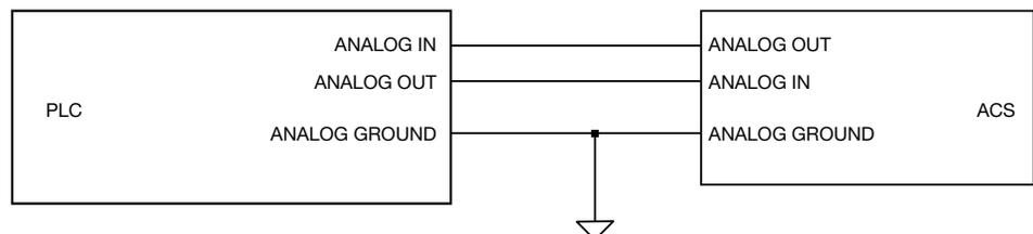
**Figure 6-10: Analog Output Equivalent Circuit**
