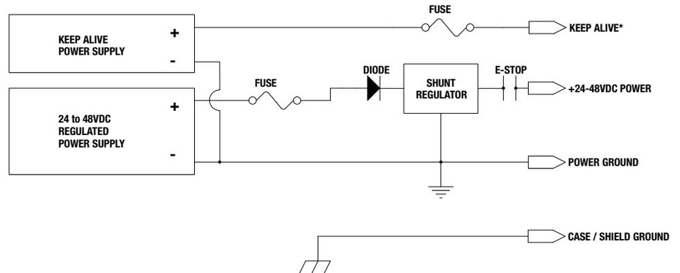
**Figure 6-16: Regulated Power Supply with Blocking Diode and Shunt Regulator**
