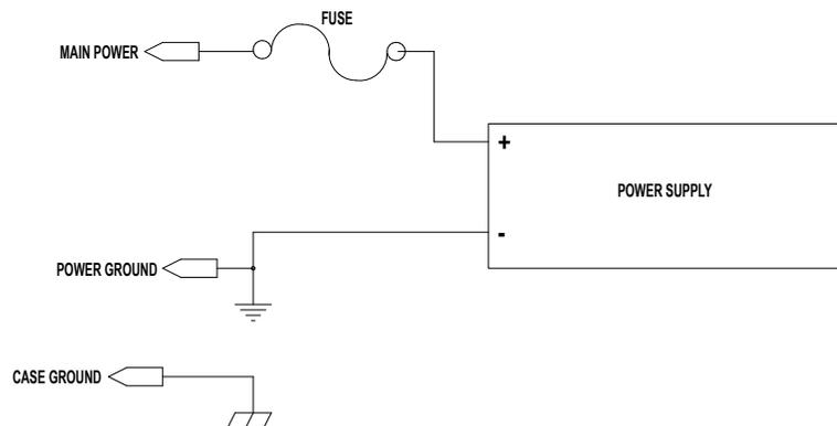
Figure 6-12: ACS Drive Single Supply – Main Power
