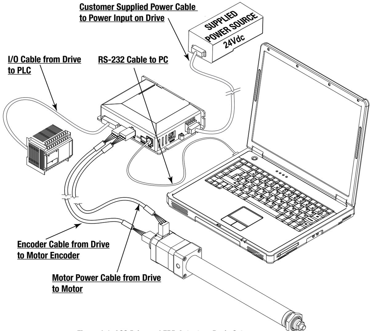
**Figure 4-1: ACS Drive and ERD Actuator– Basic Setup**
