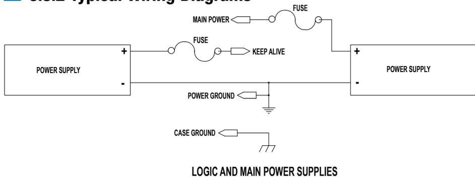
Figure 6-11: ACS Drive Logic and Main Power Supplies
