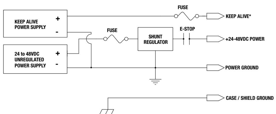
**Figure 6-14: Unregulated Power Supply Configuration with Shunt Regulator**
