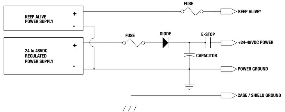
**Figure 6-15: Regulated Power Supply Configuration with Blocking Diode and Added Capacitance**
