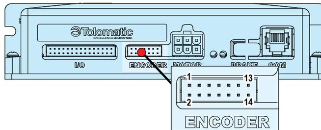
Figure 5-3: Encoder Connection on ACS Drive
