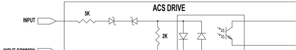
**Figure 6-1: Digital Input Circuit**
