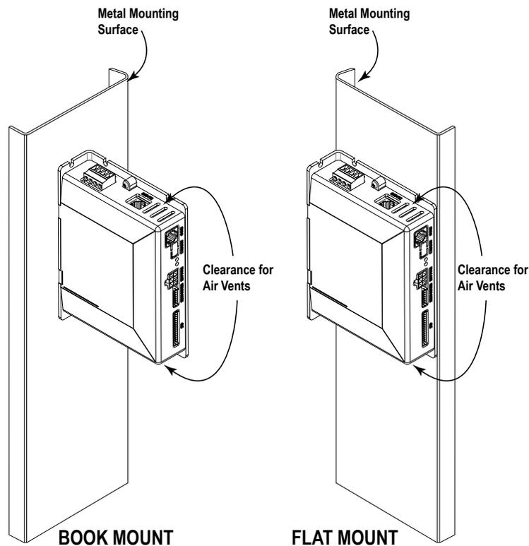
**Figure 2-2 Mounting the ACS Drive**
