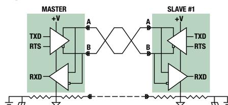
**Figure 5-10: Resistors in ground wire to limit current**
