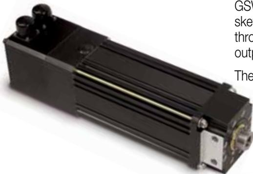
GSWA integrated motor actuator uses an 8 pole, Nd-Fe-B hollow core rotor with skewed stator laminations. This allows the magnet to remain over multiple windings throughout the weld cycle for maximum torque efficiency and consistent force output at any location along the actuator stroke.
