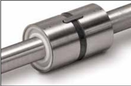
Capable of handling heavy loads. Force is transmitted via multi-threaded helical roller assemblies engaged with a fine threaded roller screw. Roller screws have exceptional loading capability based on many points of contact.
