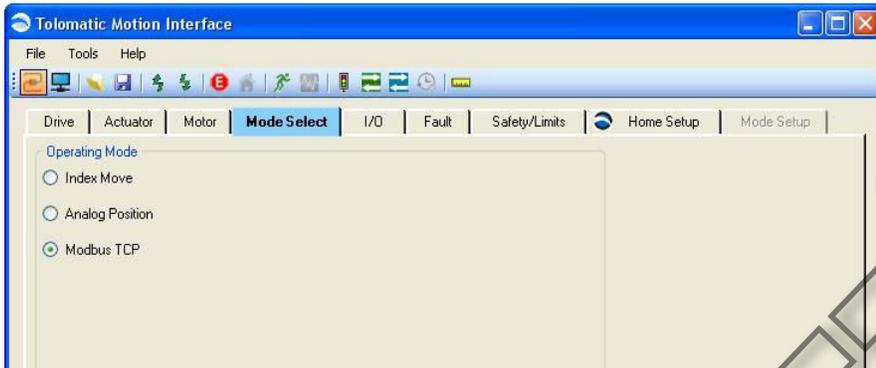
**Figure 2: Select Modbus TCP in the Mode Select Tab**
