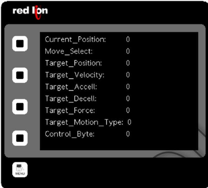
**Figure 10: Setting up a Motion Profile**
