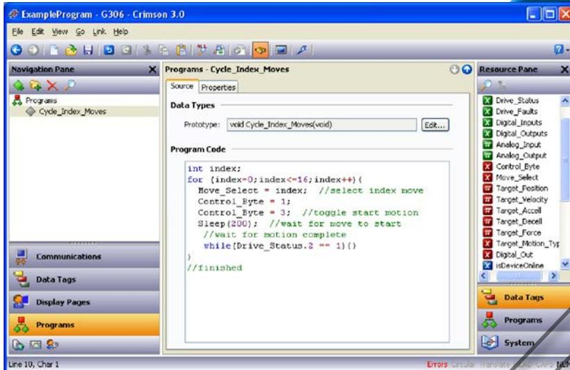
**Figure 20 : Creating a Program to Cycle Index Moves**
