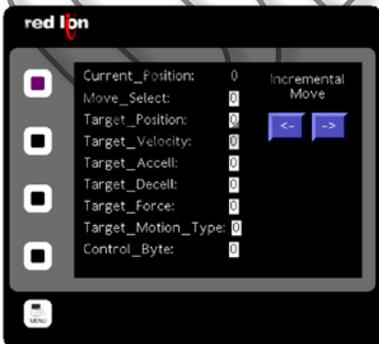
Figure 17: Adding Positive and Negative Incremental Move Buttons
