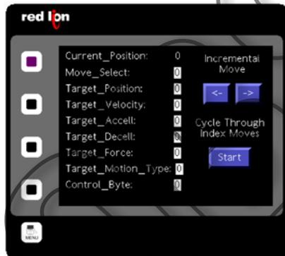
**Figure 19: Index Move Step Through Setup**
