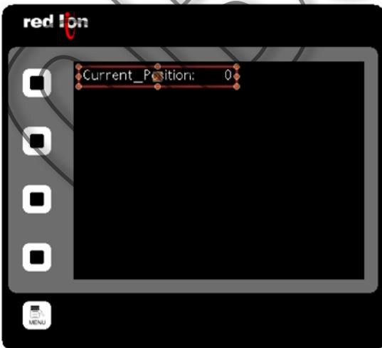
**Figure 9: Placing a Data Tag**
