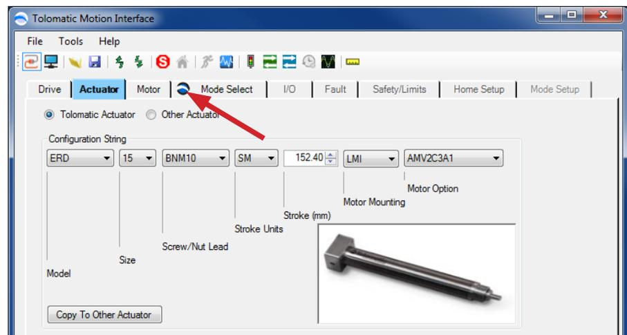
Figure 7-2: Configuring the Tolomatic Actuator Selection
