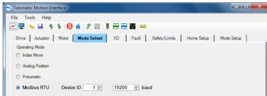
**Figure 9-6: Mode Select Tab Window - Modbus RTU**
