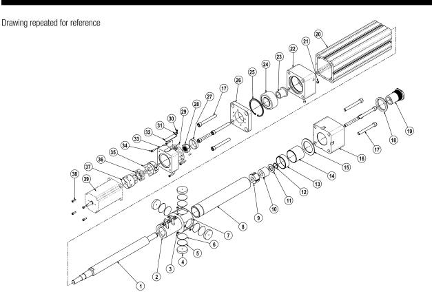
B. Align non-motor end Head to Cylinder Body with Thrust Tube extended, and then tighten Socket Head Cap Screws.
