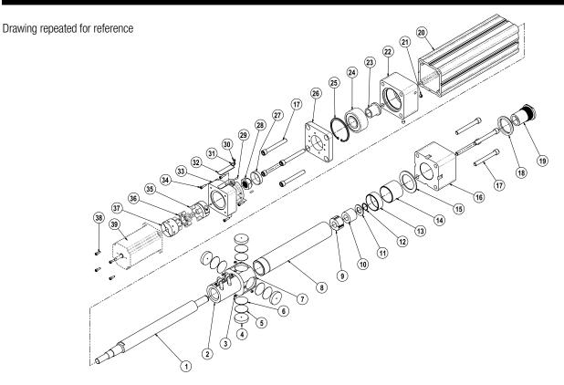
**Solid Nut/Ball Nut:** Remove the Bearing Sleeve from the Leadscrew. **Ball Nut:** \*Caution is required if removal of the Nut Assembly or Leadscrew is required. Contact the factory for available parts and procedures.
