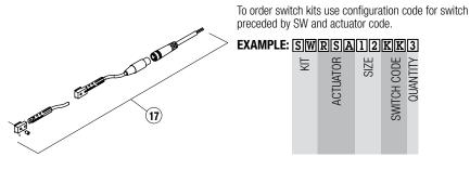
The example is for 3 Solid State NPN, Normally Open Switches with Quick-disconnect couplers. Each switch is complete with Bracket, Set Screw, Switch and mating QD cable. Note that the bracket/switch size is common and may be used on any size RSA.
