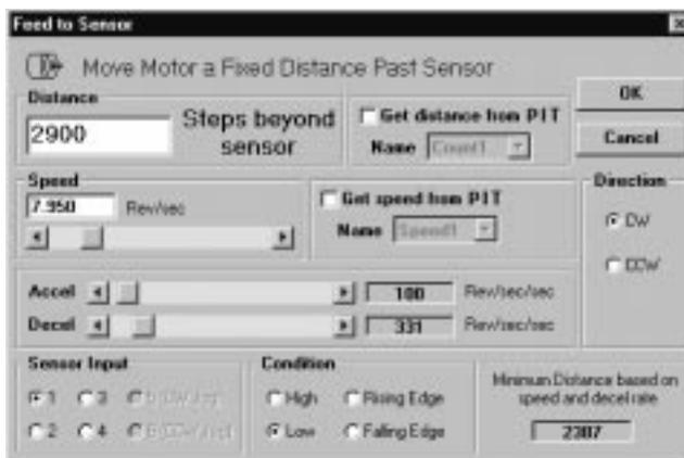
Figure 46 - FEED TO SENSOR DIALOG BOX
