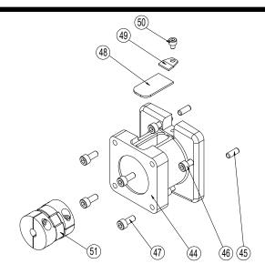
Motor Mount Kit — Model & Size Lead Screw Motor Orientation
