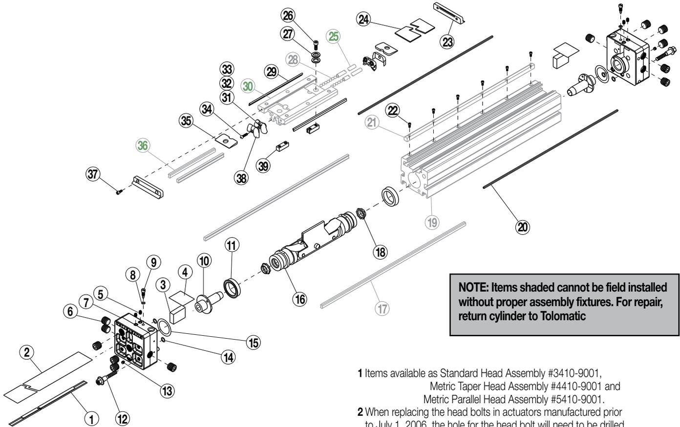
**NOTE:** Items shaded cannot be field installed without proper assembly fixtures. For repair, return cylinder to Tolomatic
