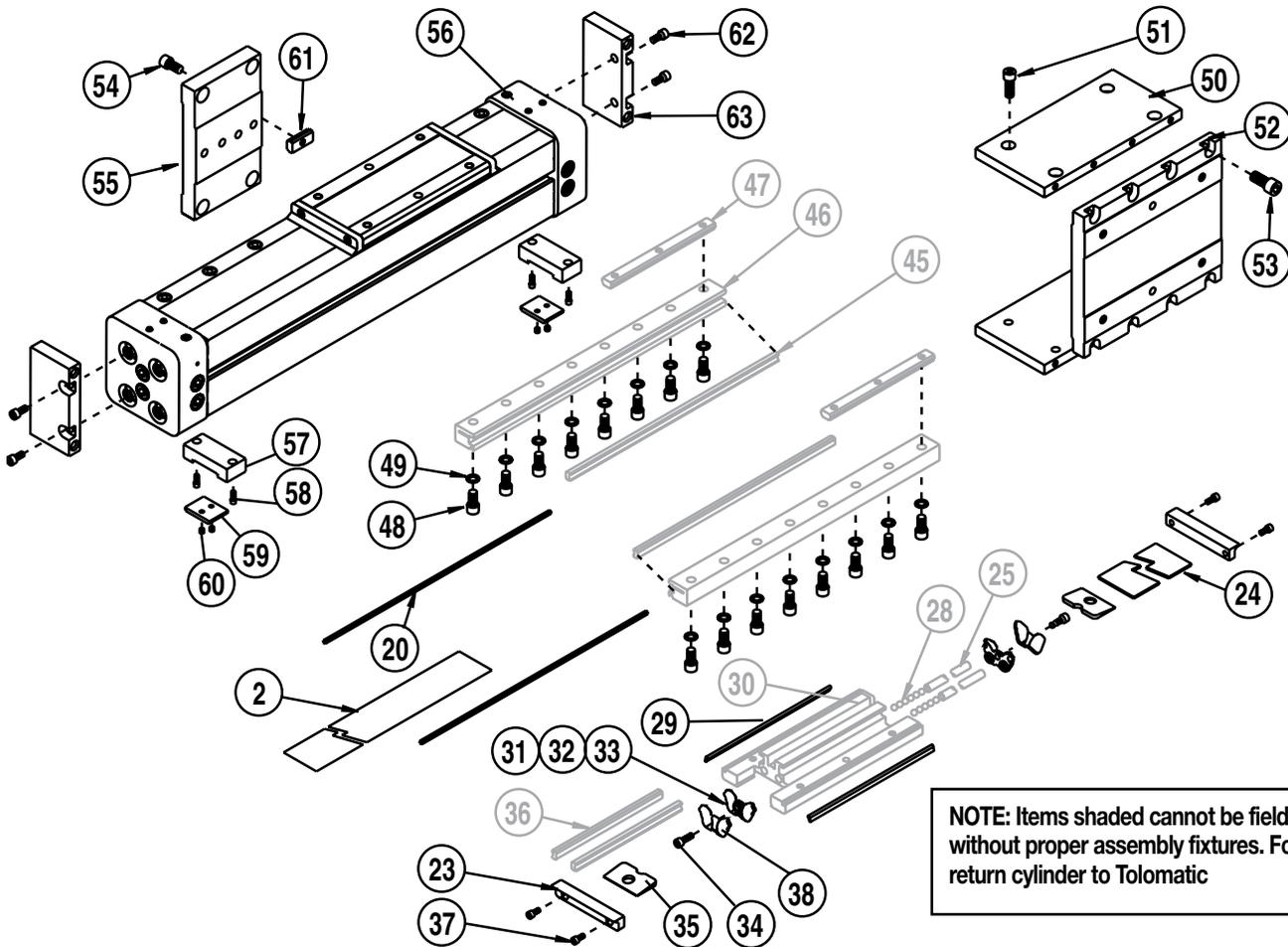
**NOTE: Items shaded cannot be field installed without proper assembly fixtures. For repair, return cylinder to Tolomatic**
