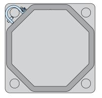
The switch bracket and switch does not extend beyond the profile of the RSX heads.
