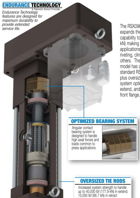
The RSX096P press actuator expands the extend force capability to 40,000 lbf (178 kN) making it well suited for applications such as pressing, riveting, clinching and many others. The RSX096P press model has all the features of the standard RSX on pages 4 & 5 plus oversized tie rods, a bearing system optimized for high force extend, and a high strength steel front flange.
