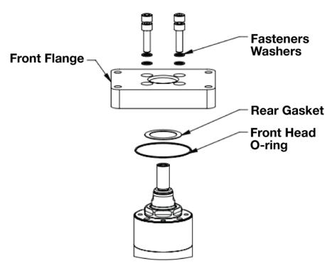
Figure 6.4: FFG option, front flange, mount feature and replaceable items
