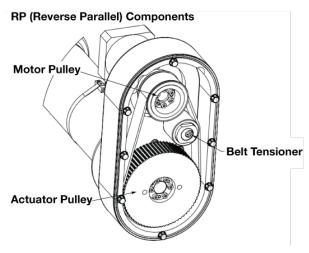
Figure 4.3: This view of the RSH reverse parallel (RP) shows the belt path in relation to the motor pulley, actuator pulley, and RP tensioner.
