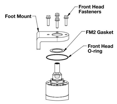
Figure 6.5: FM2 option, front flange, mount feature and replaceable items
