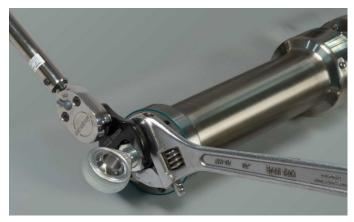
Figure 4.4: For RSH hold the thrust rod stationary using a wrench on the flats at the end of the thrust rod when attaching accessories, linkages or load to the actuator.
