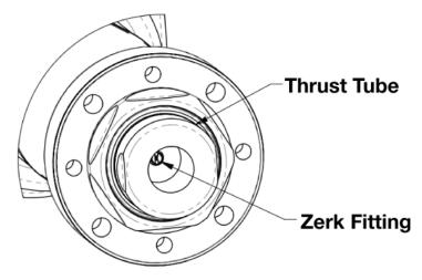
Figure 6.2: RSH zerk fitting location
