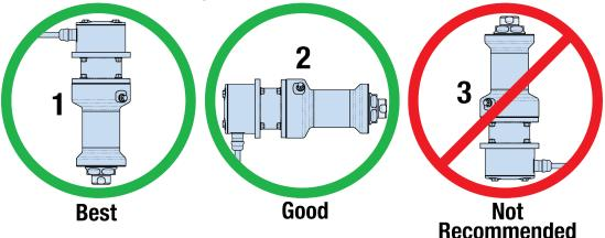
Figure 4.2: **1. & 2.** Recommended RSH thrust rod orientation is down or horizontal. **3.** Due to increased risk of contamination and ingress it is not recommended to orient the RSH actuator with the thrust rod up.
