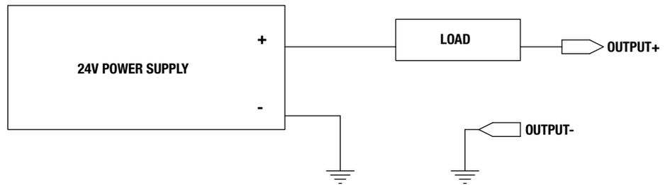
**Figure 3-15: ICR/ICM SV1P Plus Digital Output Sinking Wiring Diagram**
