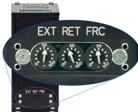
**Figure 5-5: ICR SV1B Basic Actuator Velocity and Force Controls**
