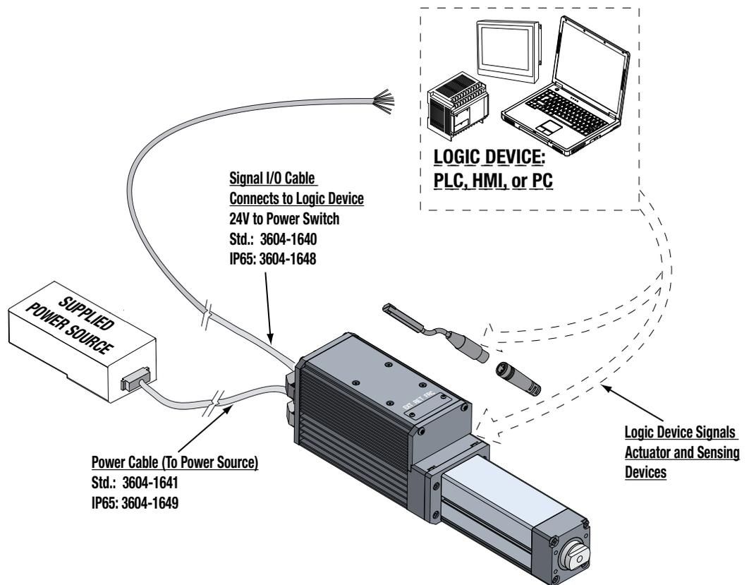
Figure 2-16: ICR SV1B Basic Actuator Setup
