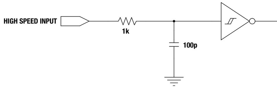
Figure 3-7: ICR/ICM SV1P Plus High Speed Digital Input Circuitry
