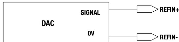
Figure 3-13: ICR/ICM SV1P Plus Analog Input Typical Wiring
