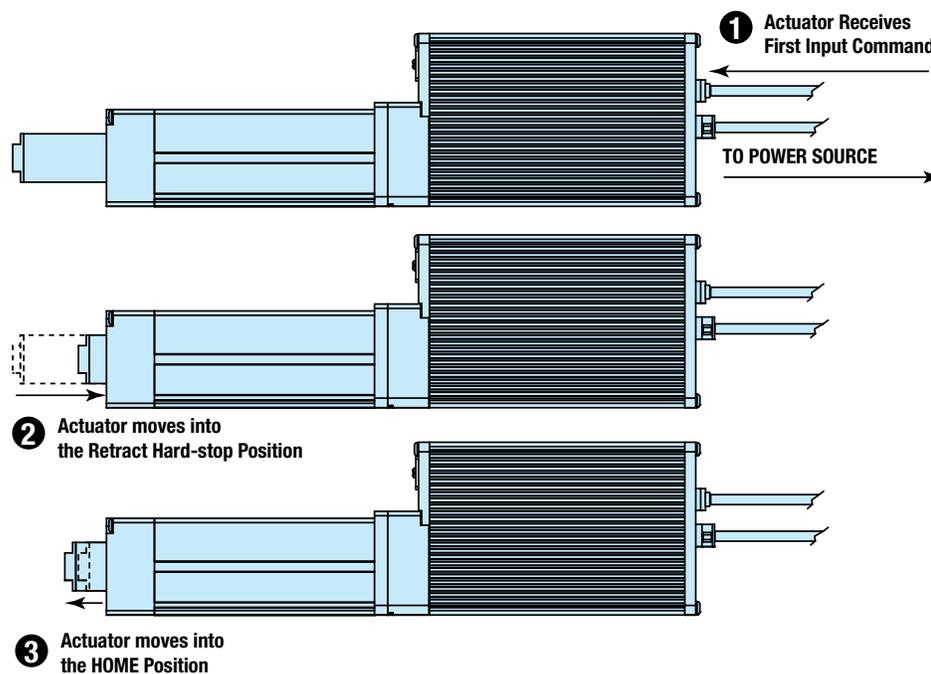
**Figure 5-2: ICR SV1B Basic Actuator Home Position**
