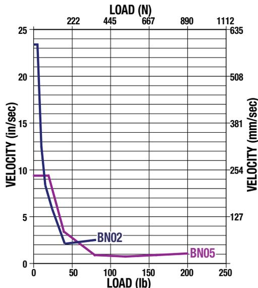
Figure 4-1: Maximum Load/Velocity of System without a Voltage Control Device
