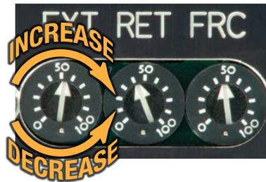
**Figure 5-6: ICR SV1B Basic Actuator Extend Velocity Potentiometer**
