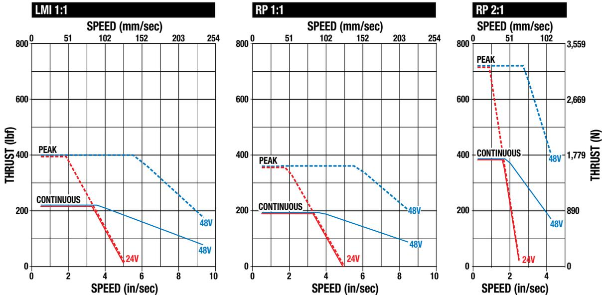
Figure 1-1: BN05 Ball Nut: Continuous and Peak Speed vs Thrust
