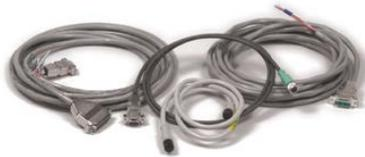
Tolomatic also provides 5-meter signal and power cables for both the ICR Basic and ICR Plus. An additional communication cable is available in either 1-meter or 5-meter lengths for the ICR Plus. All cables are available in either standard or IP65.
