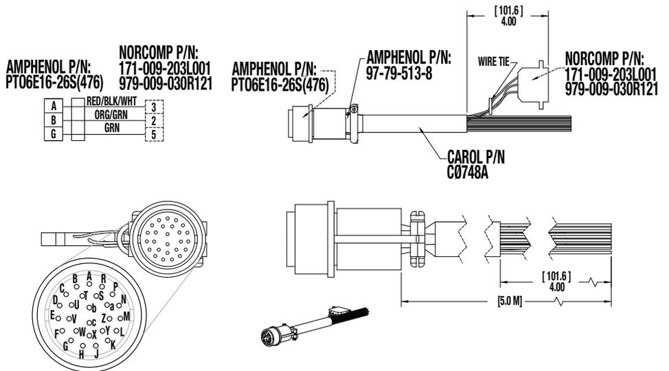
Figure 2-4: ICR SV1B Basic Actuator IP65 I/O Cable 3604-1648
