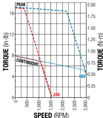
Figure 1-5: ICM Plus Motor Speed vs Torque
