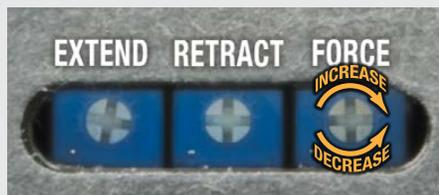
**Figure 5-12: ICR SV1B Basic Actuator Force Control Potentiometer**
