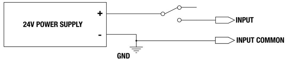
Figure 3-8: ICR/ICM SV1P Plus Source (switched) Connection
