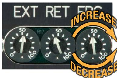
Figure 5-8: ICR SV1B Basic Actuator Force Control Potentiometer
