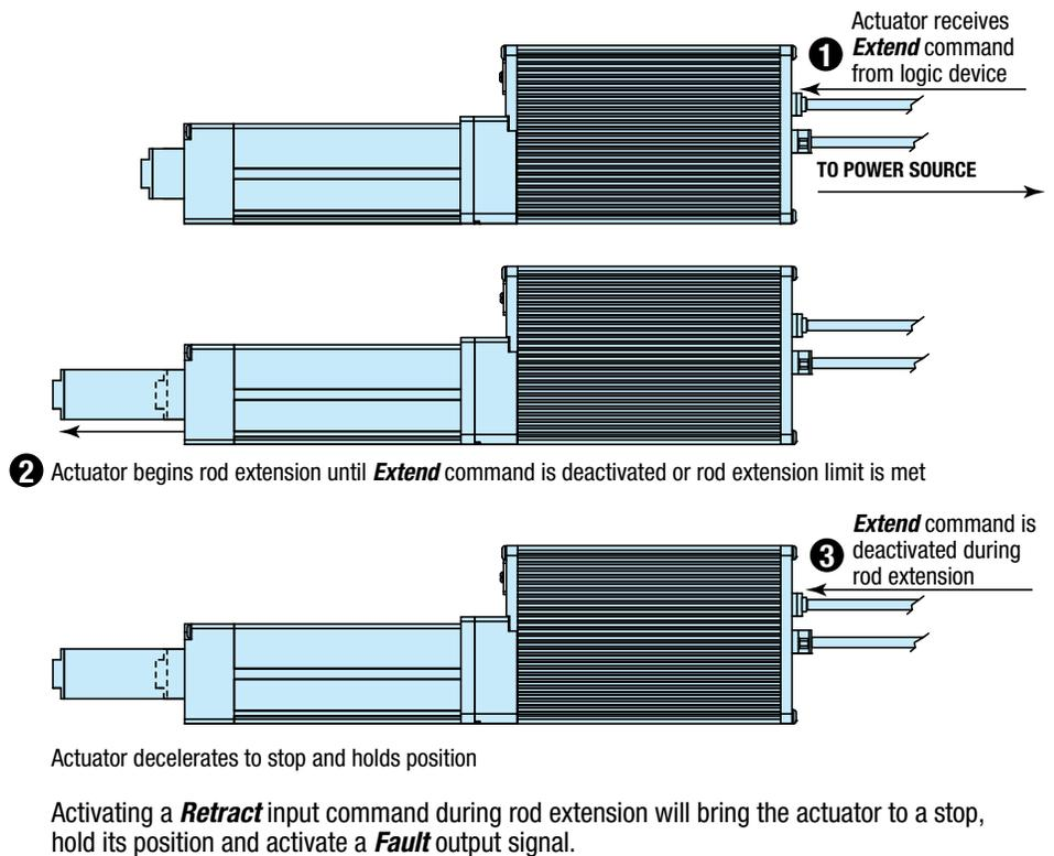
Figure 5-3: ICR SV1B Basic Actuator Extend Input Command
