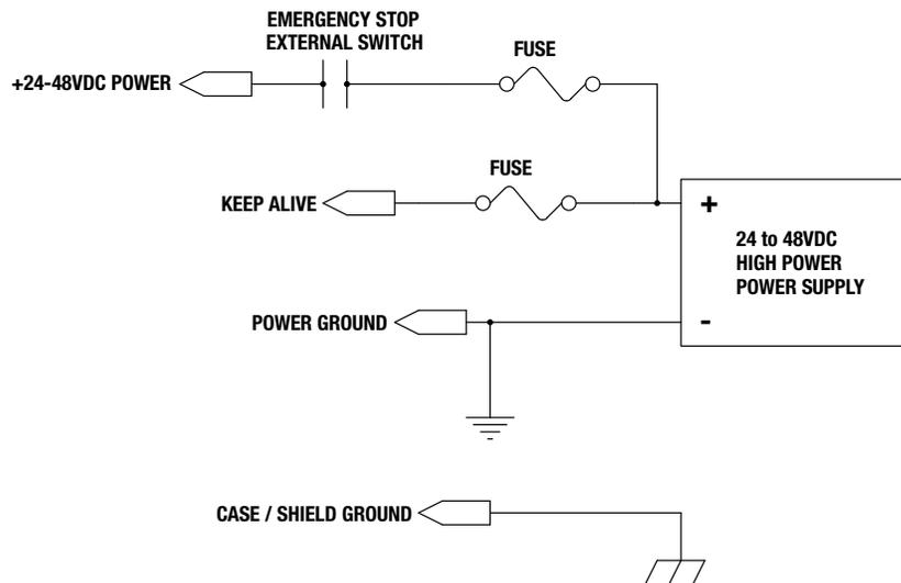
**Figure 3-19: ICR/ICM SV1P Plus Single Supply - External Cutoff Switch for Emergency Stop**
