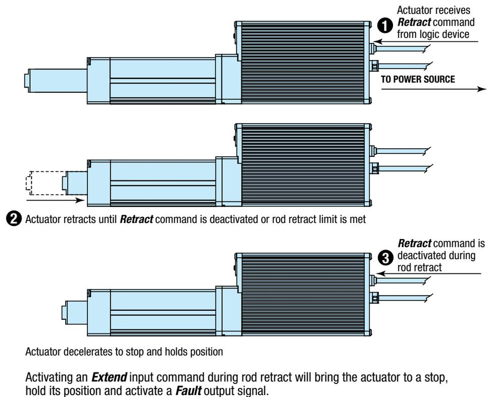
**Figure 5-4: ICR SV1B Basic Actuator Retract Input Command**
