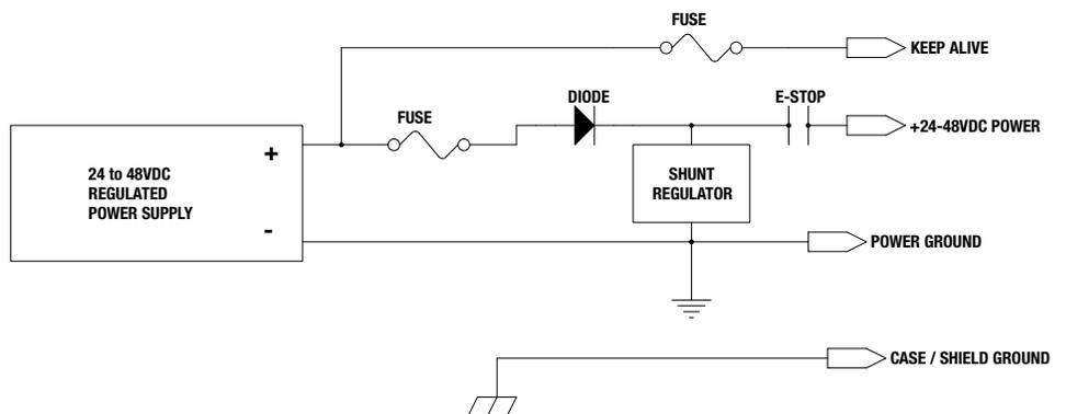
**Figure 4-4: Regulated Power Supply with Blocking Diode and Shunt Regulator**
