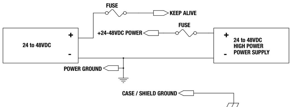
**Figure 3-17: ICR/ICM SV1P Plus Logic and Main Power Supplies**
