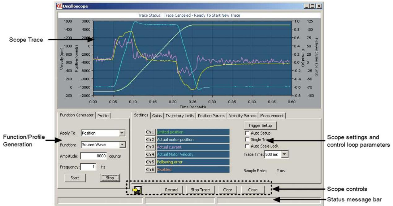
**Figure 6-14: CME 2<sup>®</sup> Scope Tool Screen**
