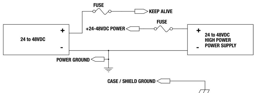
**Figure 2-13: ICR SV1B Basic Actuator Logic and Main Power Supplies**
