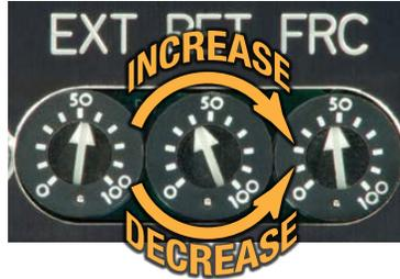
Figure 5-7: ICR SV1B Basic Actuator Retract Velocity Potentiometer
