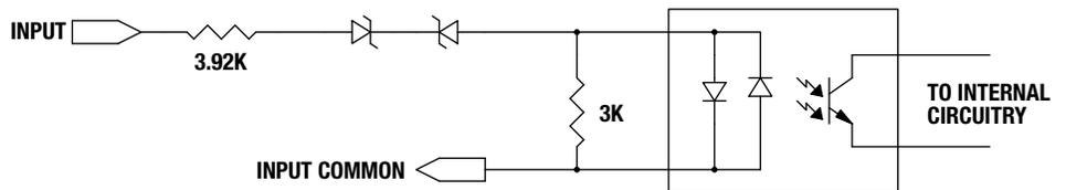
Figure 3-6: ICR/ICM SV1P Plus Isolated Interface Circuit Diagram
