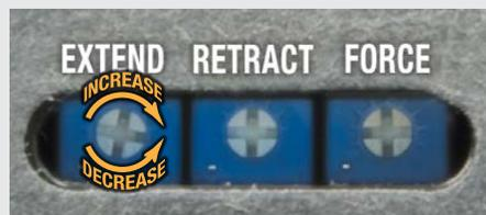
**Figure 5-10: ICR SV1B Basic Actuator Extend Velocity Potentiometer**
