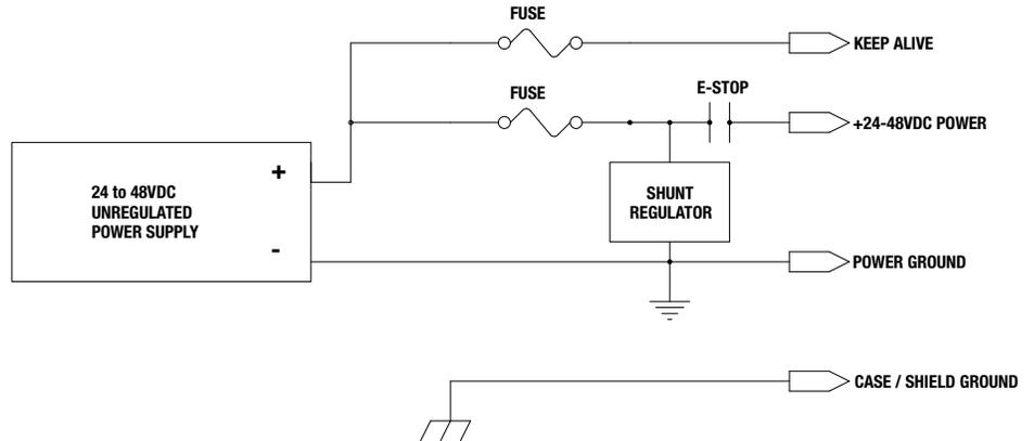
**Figure 4-2: Unregulated Power Supply Configuration with Shunt Regulator**
