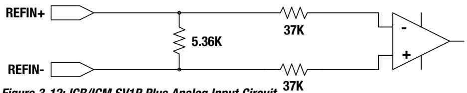
Figure 3-12: ICR/ICM SV1P Plus Analog Input Circuit
