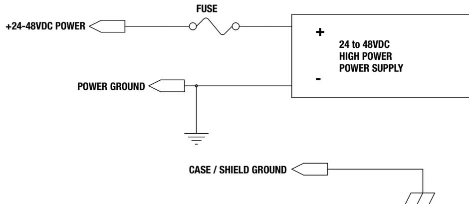
**Figure 3-18: ICR/ICM SV1P Plus Single Supply - Main Power**
