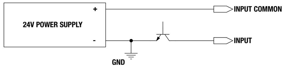
Figure 2-10: ICR SV1B Basic Actuator Input Sink (NPN) Connection
