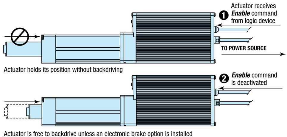
**Figure 5-1: ICR SV1B Basic Actuator Enable Input Command**
