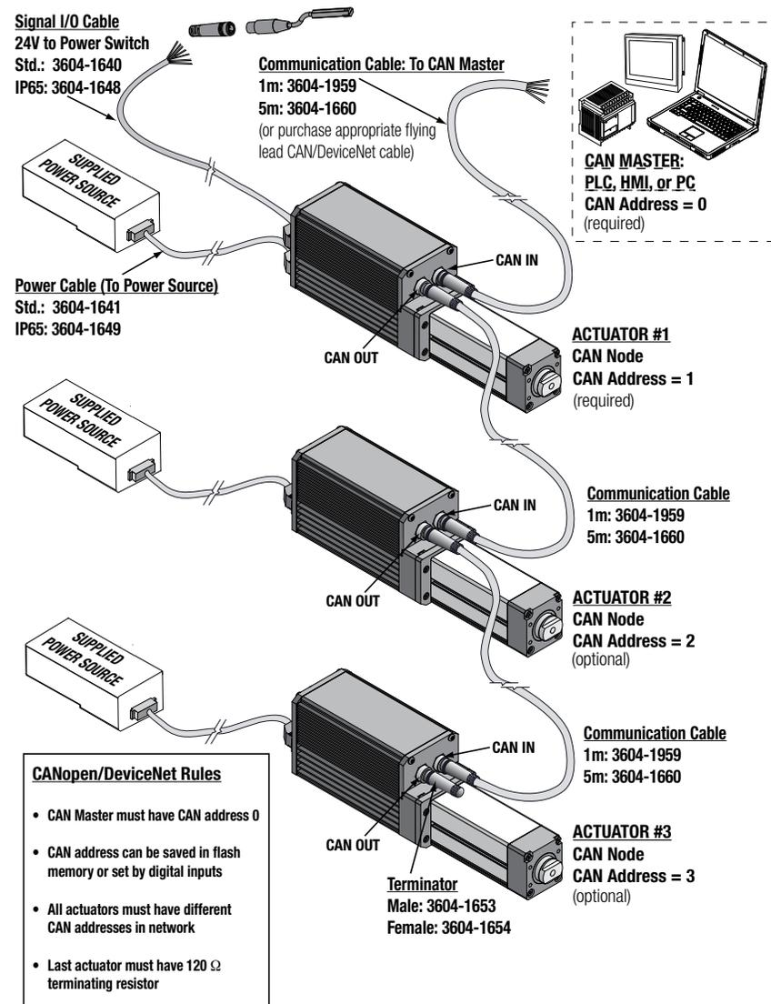
Figure 3-23: ICR/ICM SV1P Plus Multiple Actuator Setup for optional CANopen/DeviceNet Operation
