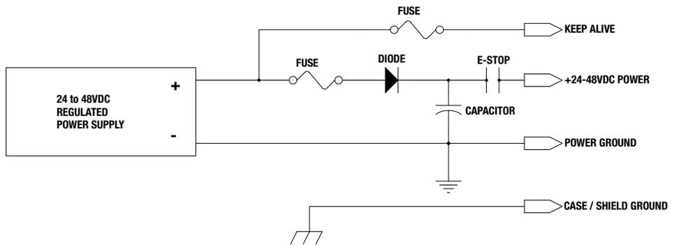
**Figure 4-3: Regulated Power Supply Configuration with Blocking Diode and Added Capacitance**
