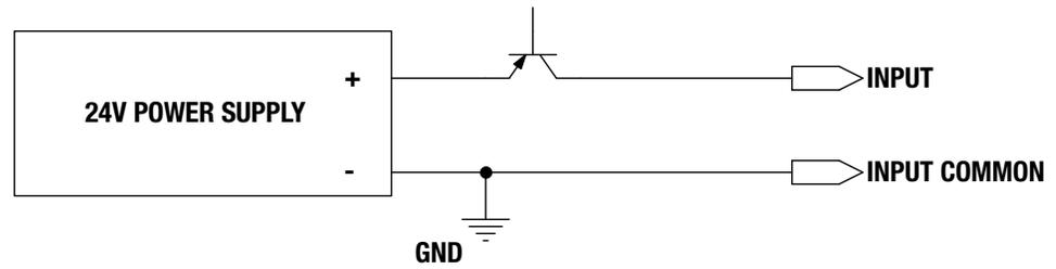
Figure 2-8: ICR SV1B Basic Actuator Input Source (PNP) Connection
