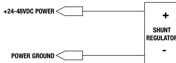
Figure 4-5: Shunt Regulator Input Wiring Diagram
