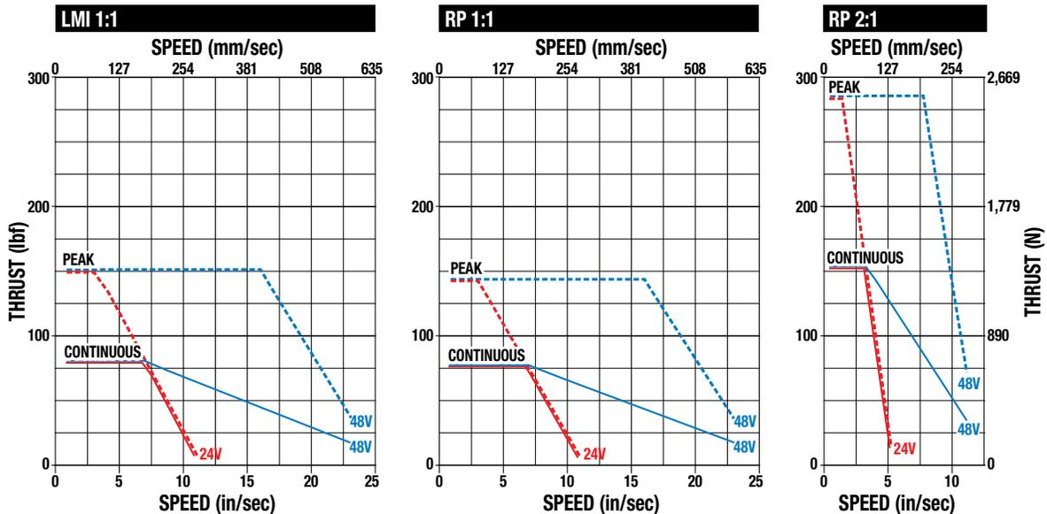
Figure 1-2: BN02 Ball Nut: Continuous and Peak Speed vs Thrust
