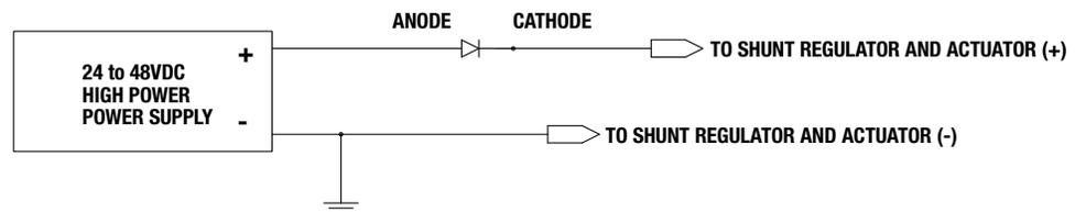
Figure 4-6: Diode Wiring Diagram
