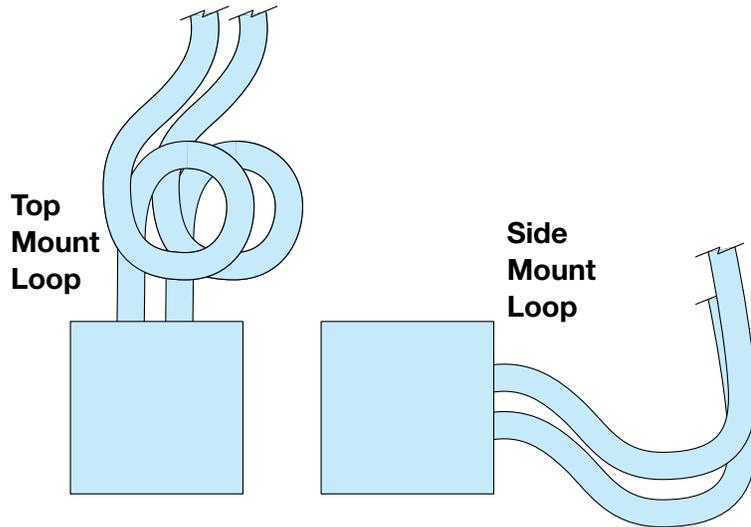
Figure 2-5: Cable Routing for Top and Side Mounted Connectors
