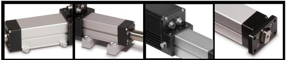
ICR SmartActuators can be mounted to an application via tube clamps, mounting plates, trunnion mounts, or front flange. The actuator also has threaded holes on the underside of the actuator heads that can be used for direct mounting.
