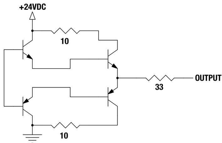
**Figure 2-11: ICR SV1B Basic Actuator Output Interface Circuit Diagram**
