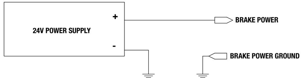
**Figure 2-12: ICR SV1B Basic Actuator Optional Electronic Brake Connection**
