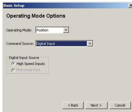
**Figure 6-10: CME 2® Basic Setup Operating Mode for Digital Input Command Source**
