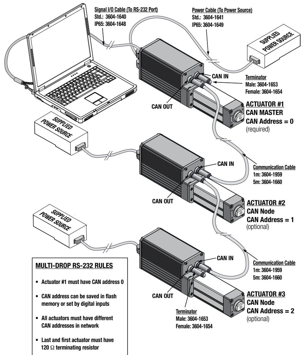
Figure 3-22: ICR/ICM SV1P Plus Multi-drop RS-232 Setup (RS-232 to optional CANopen)
