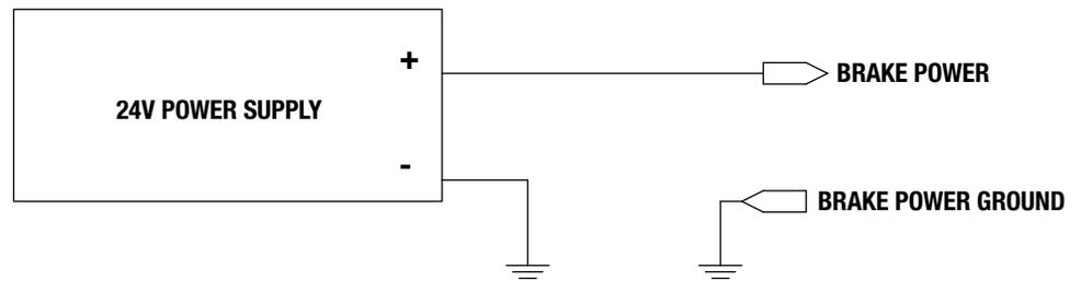
**Figure 3-20: ICR/ICM SV1P Plus Optional Electronic Brake Connection**
