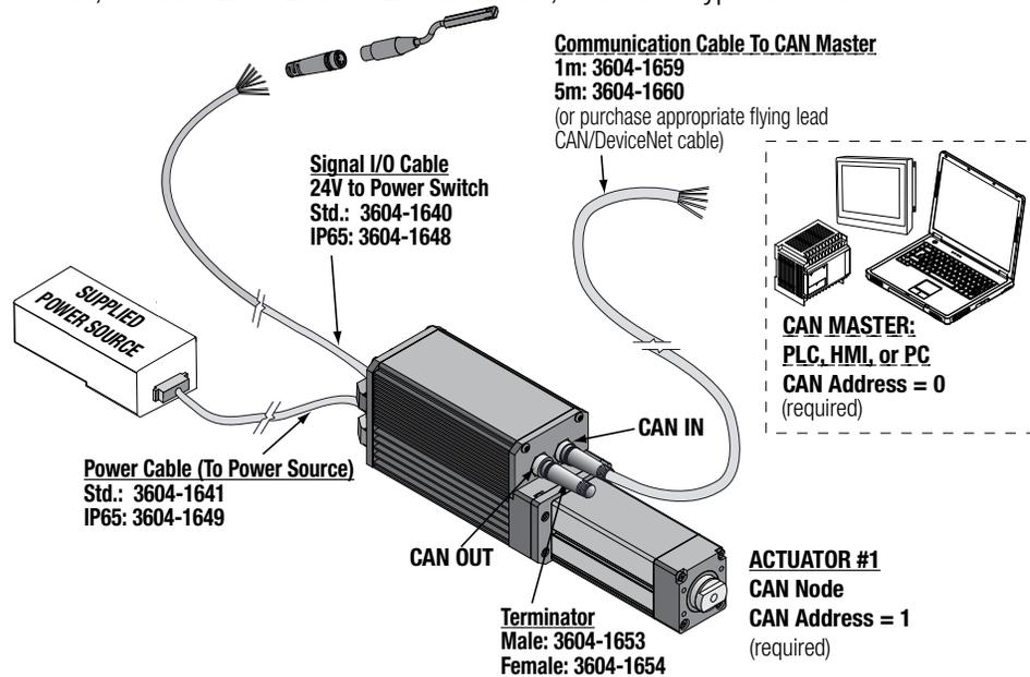
**Figure 3-21: ICR/ICM SV1P Plus Single Actuator Setup for optional CANopen Position Control**
