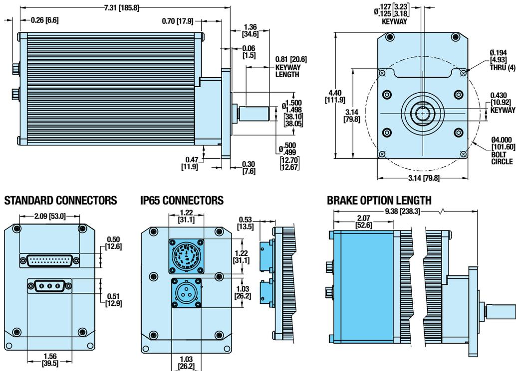
**Note:** The ICM is intended to be mounted to Tolomatic Actuators, It does NOT have a NEMA or IEC standard mount.
