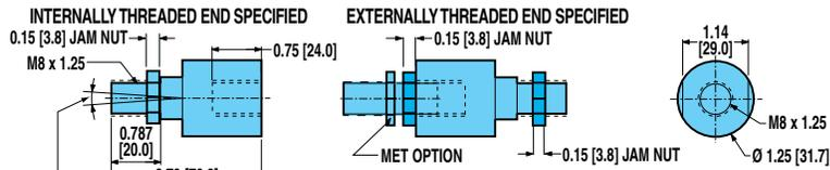
**⚠** THE ALIGNMENT COUPLER COMES WITH AN INTERNAL THREAD. IF AN EXTERNAL THREAD IS PREFERRED, THE ADDITION OF THE "MET" OPTION IS REQUIRED.
