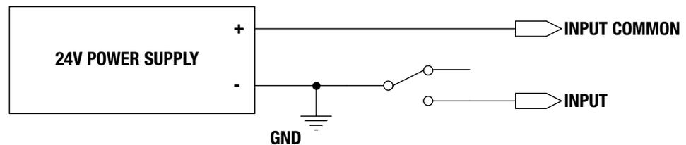
Figure 3-10: ICR/ICM SV1P Plus Sink (switched) Connection
