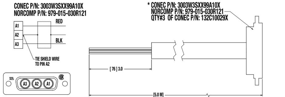
Figure 2-1: ICR SV1B Basic Actuator Standard Power Cable 3604-1641
