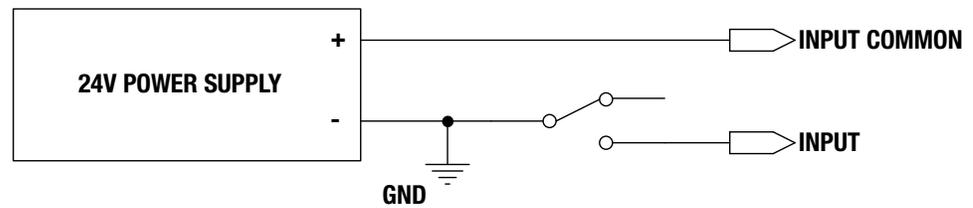
Figure 2-9: ICR SV1B Basic Actuator Input Sink (switched) Connection
