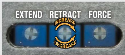
**Figure 5-11: ICR SV1B Basic Actuator Retract Velocity Potentiometer**
