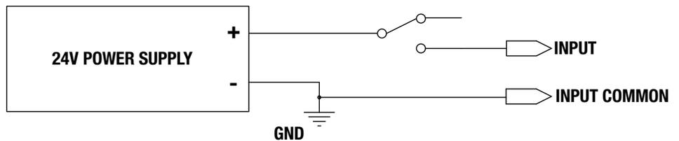
**Figure 2-7: ICR SV1B Basic Actuator Input Source (switched) Connection**
