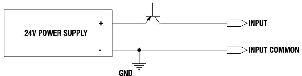
Figure 3-9: ICR/ICM SV1P Plus Source (PNP) Connection
