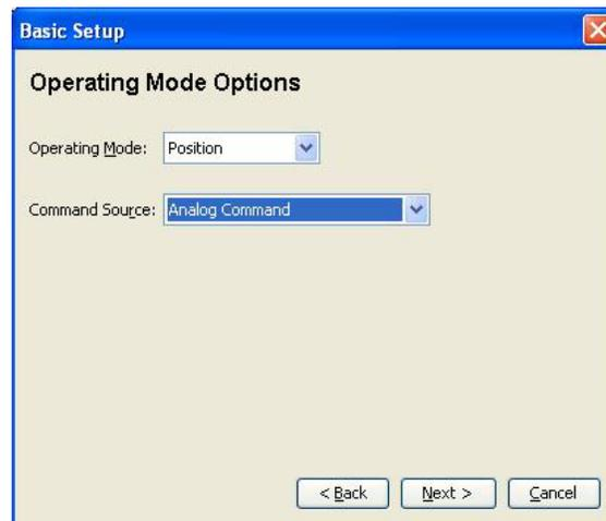
**Figure 6-9: CME 2® Basic Setup Operating Mode for Analog Command Source**
