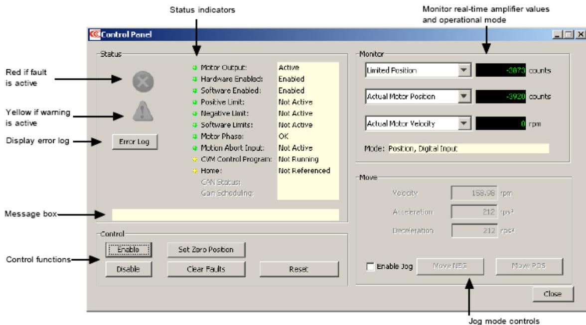
Figure 6-12: CME 2® Control Panel Features
