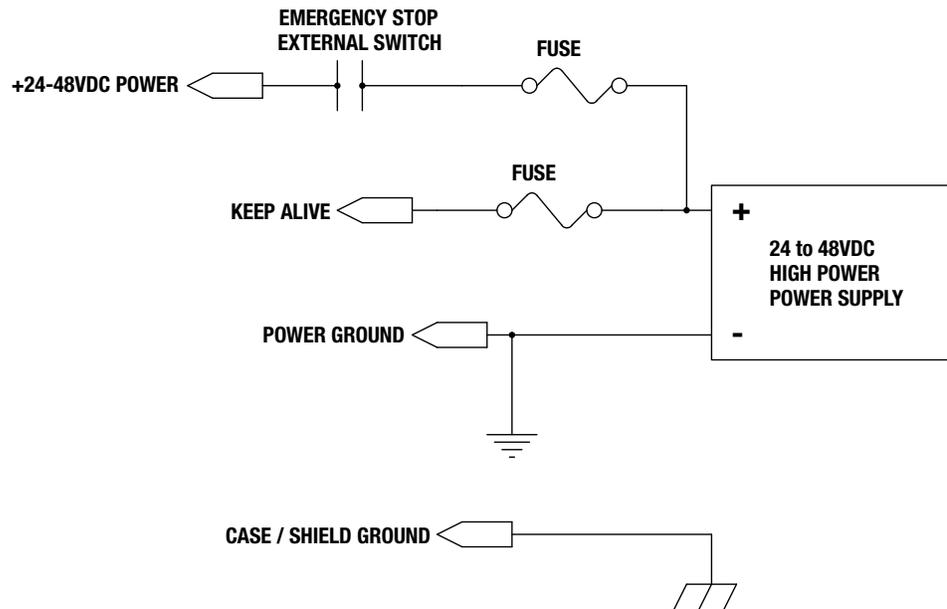
**Figure 2-15: ICR SV1B Basic Actuator Single Supply - External Cut-off Switch for Emergency Stop**
