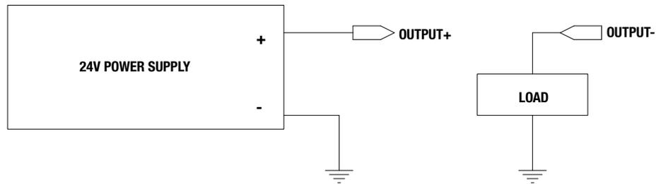
**Figure 3-16: ICR/ICM SV1P Plus Digital Output Sourcing Wiring Diagram**
