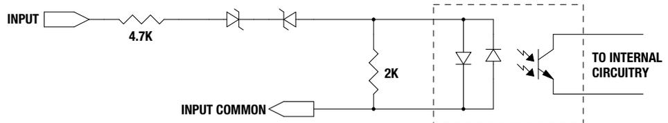
Figure 2-6: ICR SV1B Basic Actuator Interface Circuit Diagram
